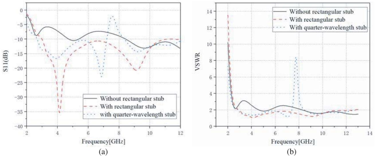
**Figure 2.** The simulated reflection coefficient and VSWR characteristic of the proposed antenna. (a)  $S_{11}$ . (b) VSWR.
