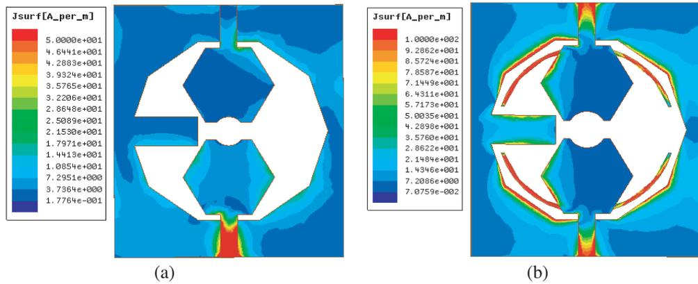
**Figure 6.** Surface current distribution of the proposed antennas.
