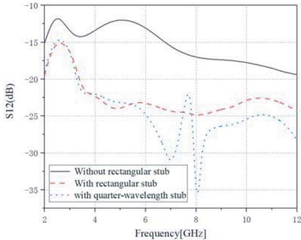
**Figure 4.** Isolation of the proposed antennas.
