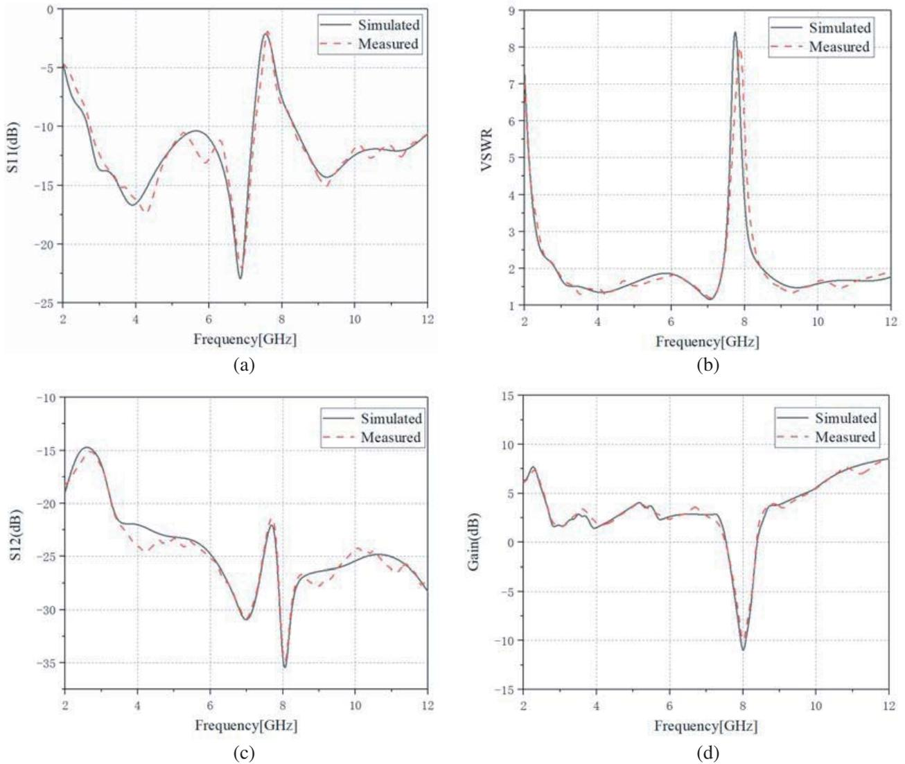
**Figure 8.** Simulated and measured of the proposed antenna, (a)  $S_{11}$ . (b) VSWR. (c)  $S_{12}$ . (d) Gain.
