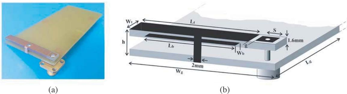
Figure 8. (a) Fabricated PIFA, (b) geometry of the proposed PIFA. The optimised design parameters are  $L_t = 35$  mm,  $W_t = 5$  mm,  $s = 4$  mm,  $L_b = 25$  mm,  $W_b = 4$  mm,  $g = 0.5$  mm,  $h = 6$  mm,  $L_g = 10$  mm,  $W_g = 40$  mm.
