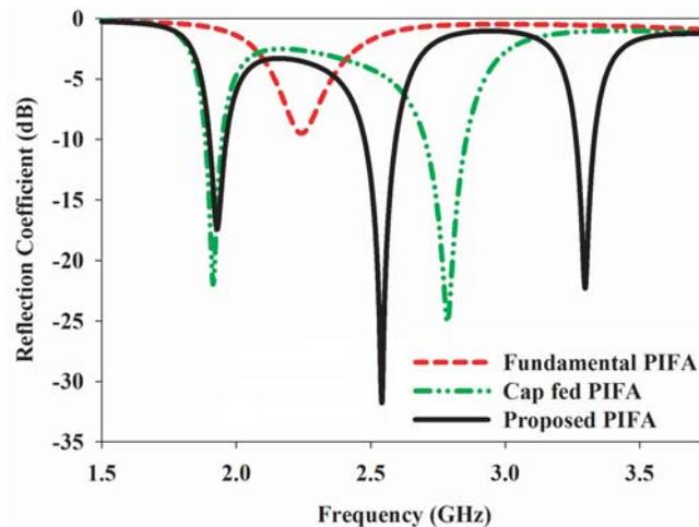
**Figure 2.** Reflection coefficients in the evolution of proposed antenna.
