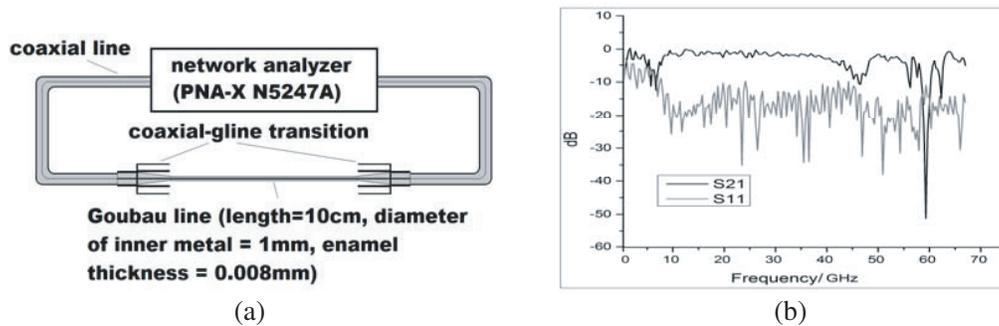
**Figure 3.** (a) Measurement setup for the proposed coaxial-G-line transition. (b) Measured  $S$ -parameters of the system involving the pair of coaxial/G-line Transitions and a Goubau line.
