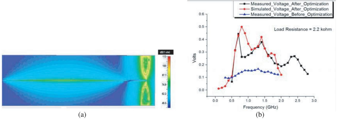
**Figure 4.** (a) Electric field distribution of the rectification section simulated using CST Studio Suite. (b) Load voltage measured against frequency when the load resistance = 2.2 kOhm and when the input power = 0 dBm.
