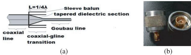
**Figure 2.** (a) Cross-sectional view of the proposed coaxial/G-line transition. (b) Photograph illustrating the proposed coaxial/G-line transitions.
