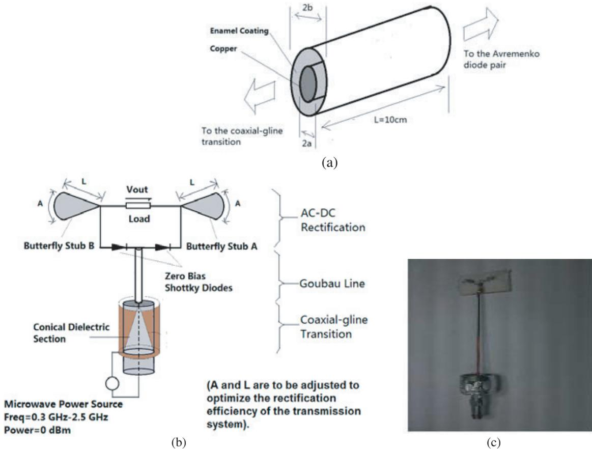
**Figure 1.** (a) Enamel coated Goubau line, with length = 10 cm, diameter of the central conductor = 1 mm and thickness of dielectric coating = 0.03 mm; (b) schematic of the proposed system for one-wire power transfer without any earth return; and (c) photograph of the final prototype.
