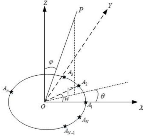
**Figure 1.** The UCA array model.
