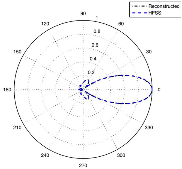
**Figure 10.** Simulated and reconstructed radiation patterns of the horn antenna.
