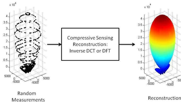
**Figure 1.** Compressive sensing algorithm for 3D radiation patterns.
