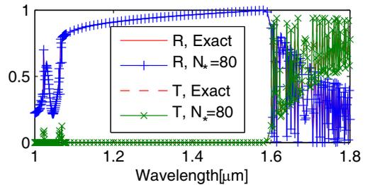
**Figure 5.** The reflection and transmission spectra for TE polarization calculated by EEM with and without mode reduction technique in the second example.  $N_* = 80$  modes are used in the mode reduction technique.
