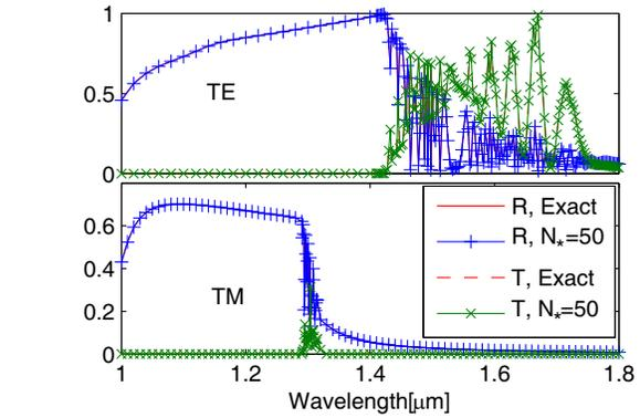
**Figure 3.** The reflection and transmission spectra calculated by EEM with and without mode reduction technique in the first example. Top figure corresponds to the TE polarization; bottom figure corresponds to the TM polarization.  $N_* = 50$  modes are used in the mode reduction technique.
