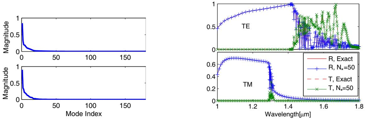
**Figure 2.** The absolute value of the first 180 elements in the first column of  $\mathbf{S}(x_1^-, x_2^+)$  in the first example with wavelength  $\lambda = 1.55 \mu\text{m}$ . Top and bottom pictures correspond to TE and TM polarizations, respectively.
