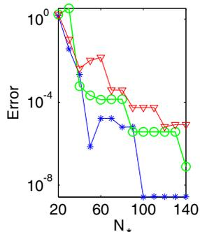
**Figure 6.** Error of reflection computed by EEM with mode reduction technique with different  $N_*$  and  $N$  in the second example at wavelength  $\lambda = 1.62 \mu\text{m}$  for TE polarization. Blue star for  $N = 280$ , green circle for  $N = 560$  and red triangle for  $N = 1120$ .
