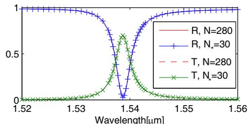
**Figure 7.** The reflection and transmission spectra of the defect waveguide calculated by EEM with and without mode reduction technique for TE polarization in the third example.  $N_* = 30$  modes are used in the mode reduction technique.
