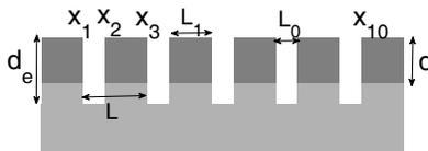
**Figure 1.** A schematic view of a piecewise uniform waveguide with 5 grooves ( $m = 10$ ). The thickness of waveguide core is  $d$  and the deepness of grooves is  $d_e$ . The width of the “teeth” and “grooves” are  $L_1$  and  $L_0$ , respectively. The period is  $L = L_0 + L_1$ .
