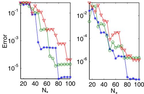
**Figure 4.** Error of transmission and reflection computed by EEM with mode reduction technique for different  $N_*$  and  $N$  in the first example. Left figure is for transmission of TE polarization at wavelength  $\lambda = 1.48 \mu\text{m}$ ; right figure is for reflection of TM polarization at wavelength  $\lambda = 1.29 \mu\text{m}$ . Blue star, green circle and red triangle are for  $N = 180$ ,  $N = 360$  and  $N = 720$ , respectively.
