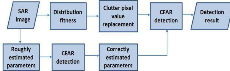
**Figure 1.** Flow of the CFAR detection algorithm.
