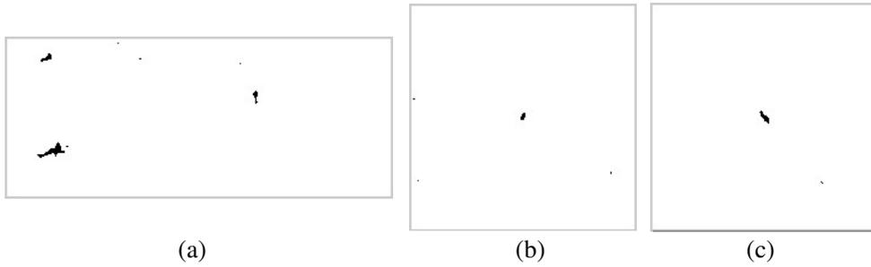
**Figure 7.** Detection results with correlation-based joint CFAR for SAR images without subsequent morphological operations on binary images. (a) Detection result for image Figure 3(a), ( $P_{fa} = 10^{-7}$ ). (b) Detection result for image Figure 4(a), ( $P_{fa} = 10^{-9}$ ). (c) Detection result for image Figure 5(a), ( $P_{fa} = 10^{-9}$ ).
