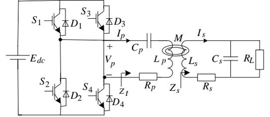
**Figure 2.** An SP-type IPT system with full-bridge inverter circuit.
