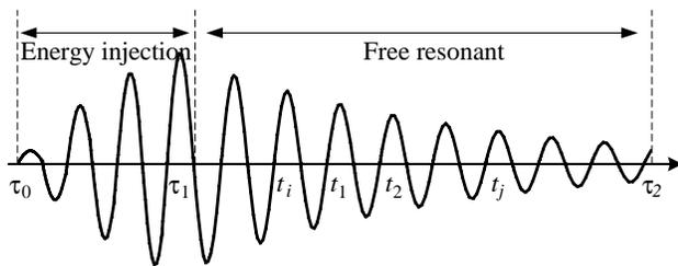
**Figure 3.** Energy injection and the free resonant mode.
