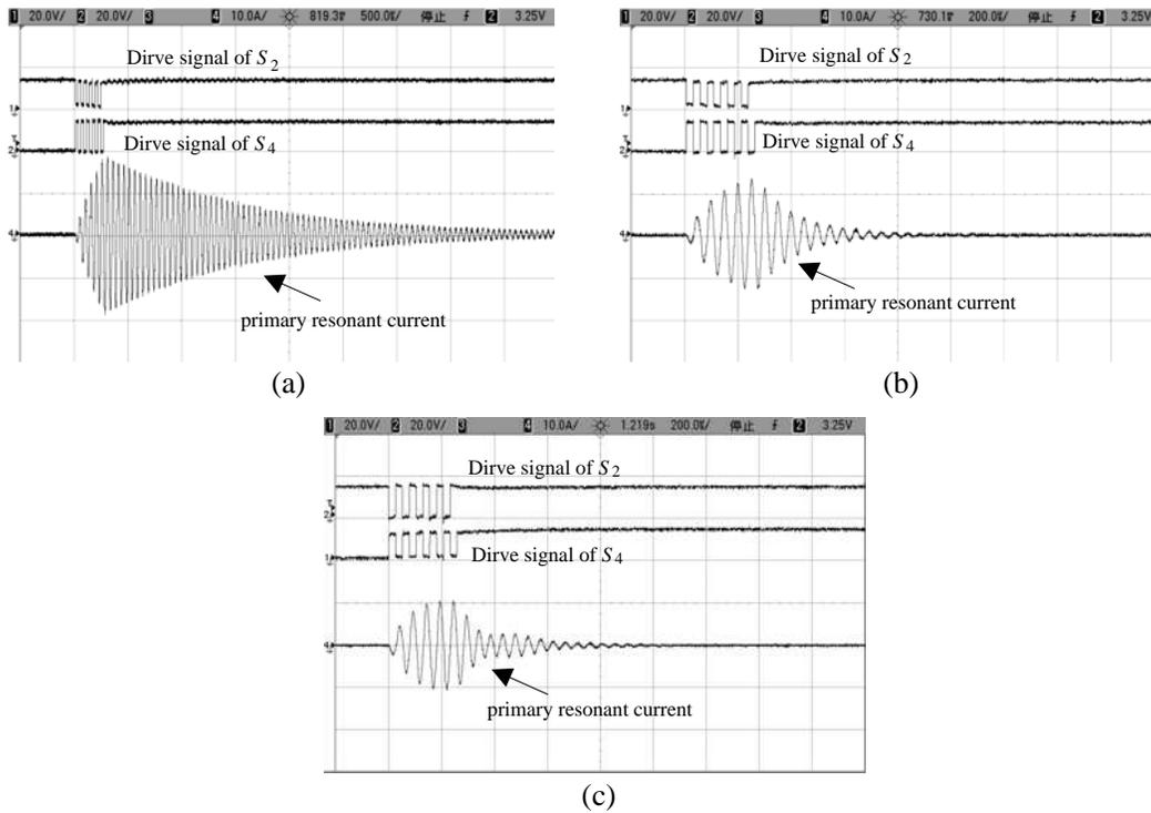
**Figure 8.** Experimental waveforms of energy injection and free resonant mode with different load conditions. (a)  $M = 0$ . (b)  $R_L = 100 \Omega$  and  $M = 40 \mu\text{H}$ . (c)  $R_L = 200 \Omega$  and  $M = 40 \mu\text{H}$ .
