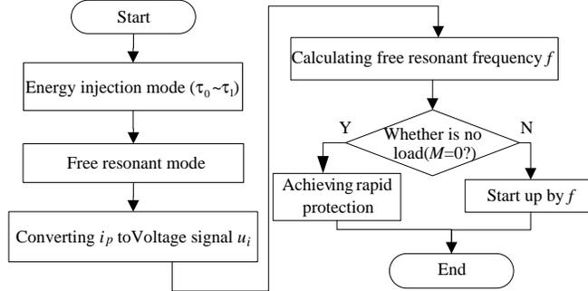
**Figure 5.** Flowchart of the startup frequency setting process.
