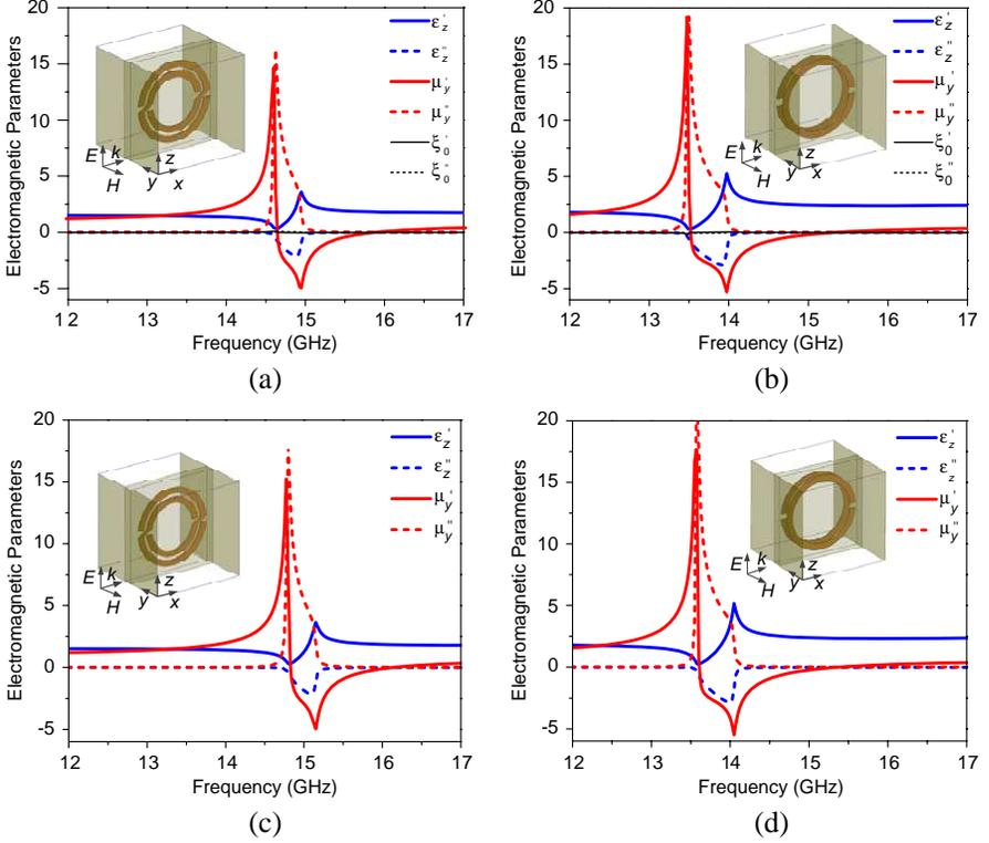
**Figure 6.** Retrieval results of the NB-SRR and BC-SRR using the proposed technique are shown in (a) and (b). As a comparison, the results obtained from the standard retrieval method [5] are given in (c) and (d).
