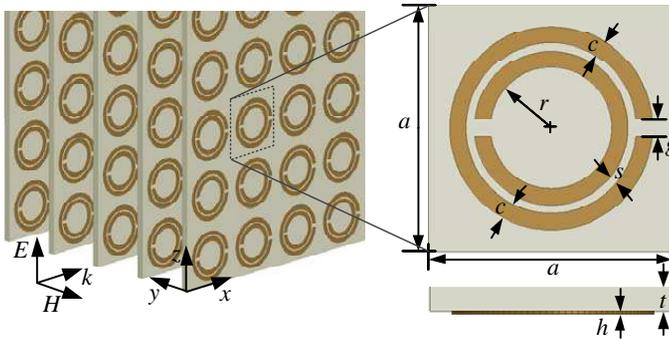
**Figure 1.** The SRRs printed on the substrates with the metallization in yellow. A plane wave is incident in the  $x$  direction polarized in the  $z$  direction. For numerical calculation, we choose the dimensions as  $a = 3$  mm,  $r = 0.74$  mm,  $c = 0.2$  mm,  $s = 0.1$  mm,  $g = 0.2$  mm,  $t = 0.3$  mm,  $h = 35 \mu\text{m}$  and assume the permittivity of the substrate is  $\epsilon_0$  for convenience.
