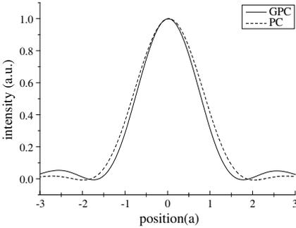
**Figure 5.** Intensities on the image plane versus the distance from the central maximum. The solid line is for the GPC and the dashed line is for the ordinary PC ( $r = 0.42a$ ).
