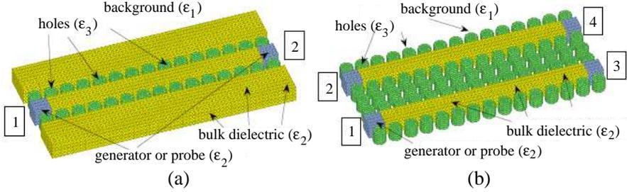
**Figure 4.** Modelling two composite dielectric structures with LEGO: (a) single waveguide and (b) two parallel waveguides comprised of “defects.” (For visualization’s sake the surface of the bricks that embed the cylindrical holes is not displayed.)
