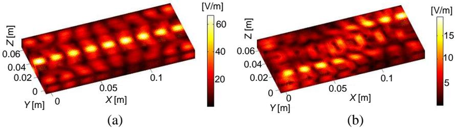
**Figure 5.** Computed  $|\mathbf{E} \times \hat{\mathbf{n}}|$  for the structures of Fig. 4: (a) single waveguide with generator brick at port 1 (port 2) on (off); (b) two waveguides with generator brick at port 1 (ports 2, 3, 4) on (off).
