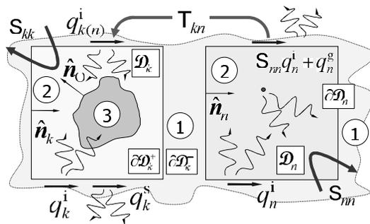
**Figure 1.** For defining passive ( $\mathcal{D}_k$ ) and generator ( $\mathcal{D}_n$ ) LEGO bricks along with scattering and transfer operators, plus equivalent incident ( $q_{k,n}^i$ ), scattered ( $q_{k,n}^s$ ) and generator ( $q_n^g$ ) currents. The labels ①, ② and ③ denote background, host and object medium, respectively.
