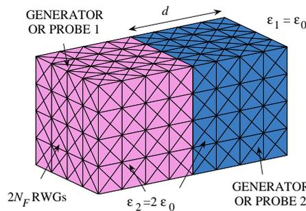
**Figure 2.** For validation of generator/probe LEGO bricks: a dielectric slab ( $\epsilon_2$ ), immersed in free space ( $\epsilon_1$ ), is modelled with  $N_D = 2$  cubic bricks. An elementary dipole of moment  $\mathbf{p}_e$  or  $\mathbf{p}_h$  is located at each brick's center. *Data:*  $d = 1$  cm,  $2N_F = 1152$ ,  $n_A = 30$ ,  $f \in [5, 7]$  GHz.
