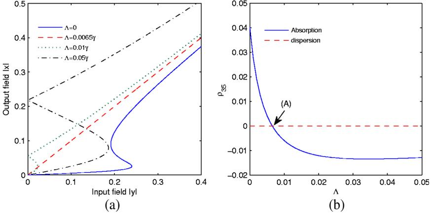
**Figure 4.** (a) The OB behavior of the system for  $\Lambda = 0$  (solid),  $\Lambda = 0.0065\gamma$  (dashed),  $0.01\gamma$  (dotted),  $0.05\gamma$  (dash-dotted). (b) Absorption (solid) and dispersion (dashed) of probe field versus incoherent pumping rate. The coupling Rabi frequencies are  $g_{13} = g_{23} = g_{14} = g_{24} = 2\gamma$ . The other parameters are same as in Fig. 2.
