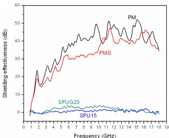
**Figure 3.** Shielding effectiveness in the 1–18 GHz range.
