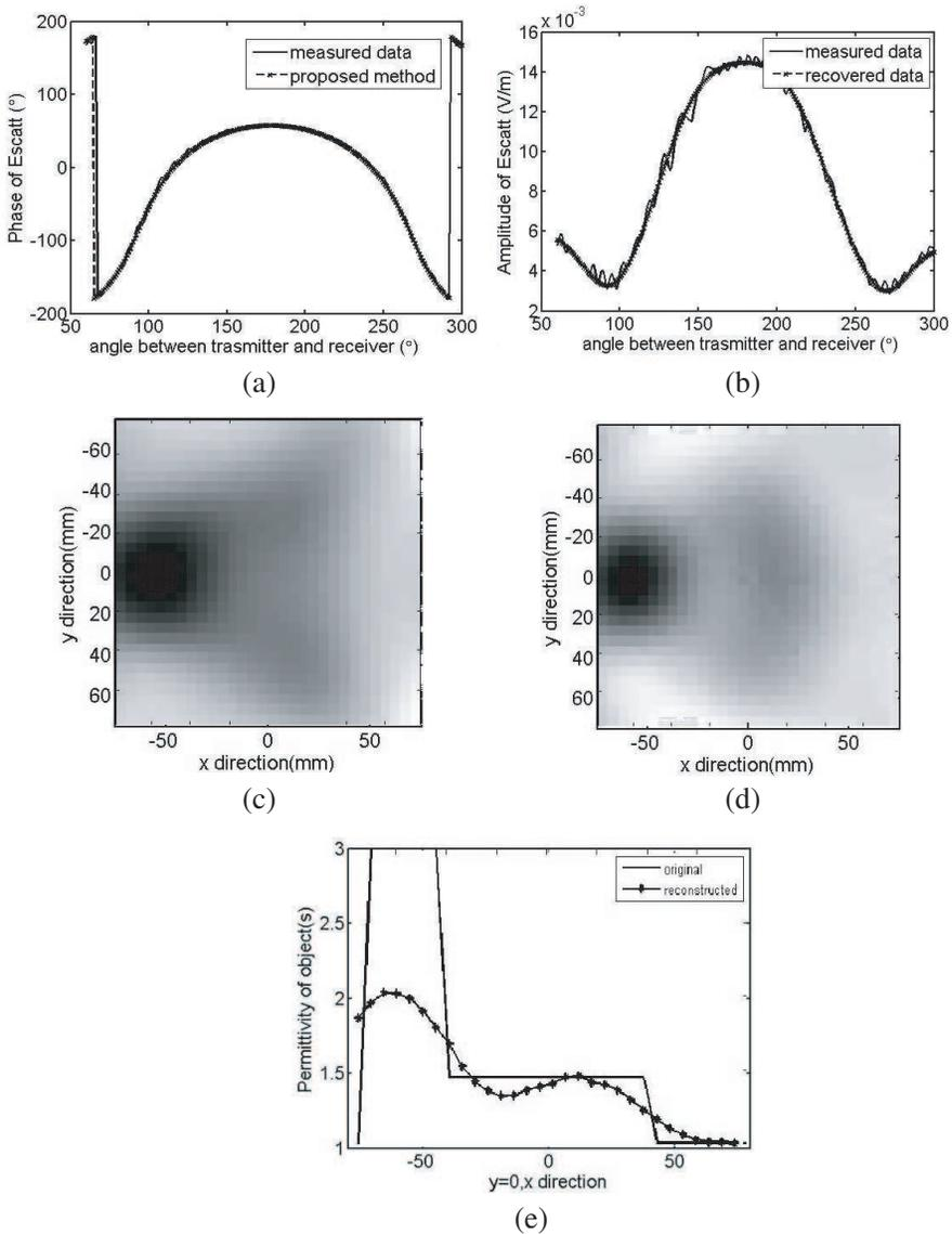
**Figure 6.** The reconstruction for probed objects shown in Fig. 2(b): (a) phase of the scattered field ( $\theta_s = 0^\circ$ ), (b) amplitude of the scattered field ( $\theta_s = 0^\circ$ ), (c) contrast map of the objects estimated by radiating equivalent current, (d) contrast map of the objects estimated by all equivalent current, (e) relative permittivity on the line  $y = 0$ .
