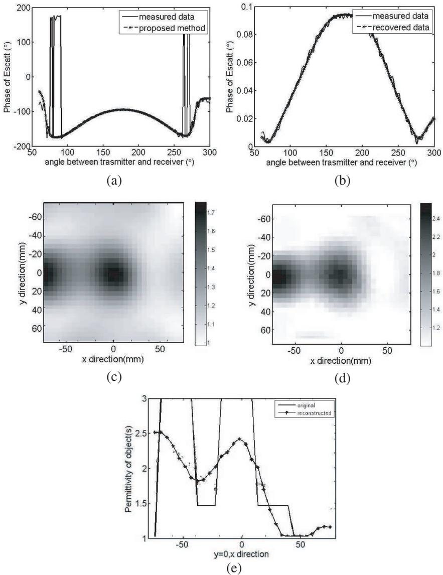
**Figure 7.** The reconstruction for the objects shown in Fig. 2(c): (a) phase of the scattered field ( $\theta_s = 0^\circ$ ), (b) amplitude of the scattered field ( $\theta_s = 0^\circ$ ), (c) contrast map of the objects estimated by radiating equivalent current, (d) contrast map of the objects estimated by all equivalent current, (e) relative permittivity on the line  $y = 0$ .
