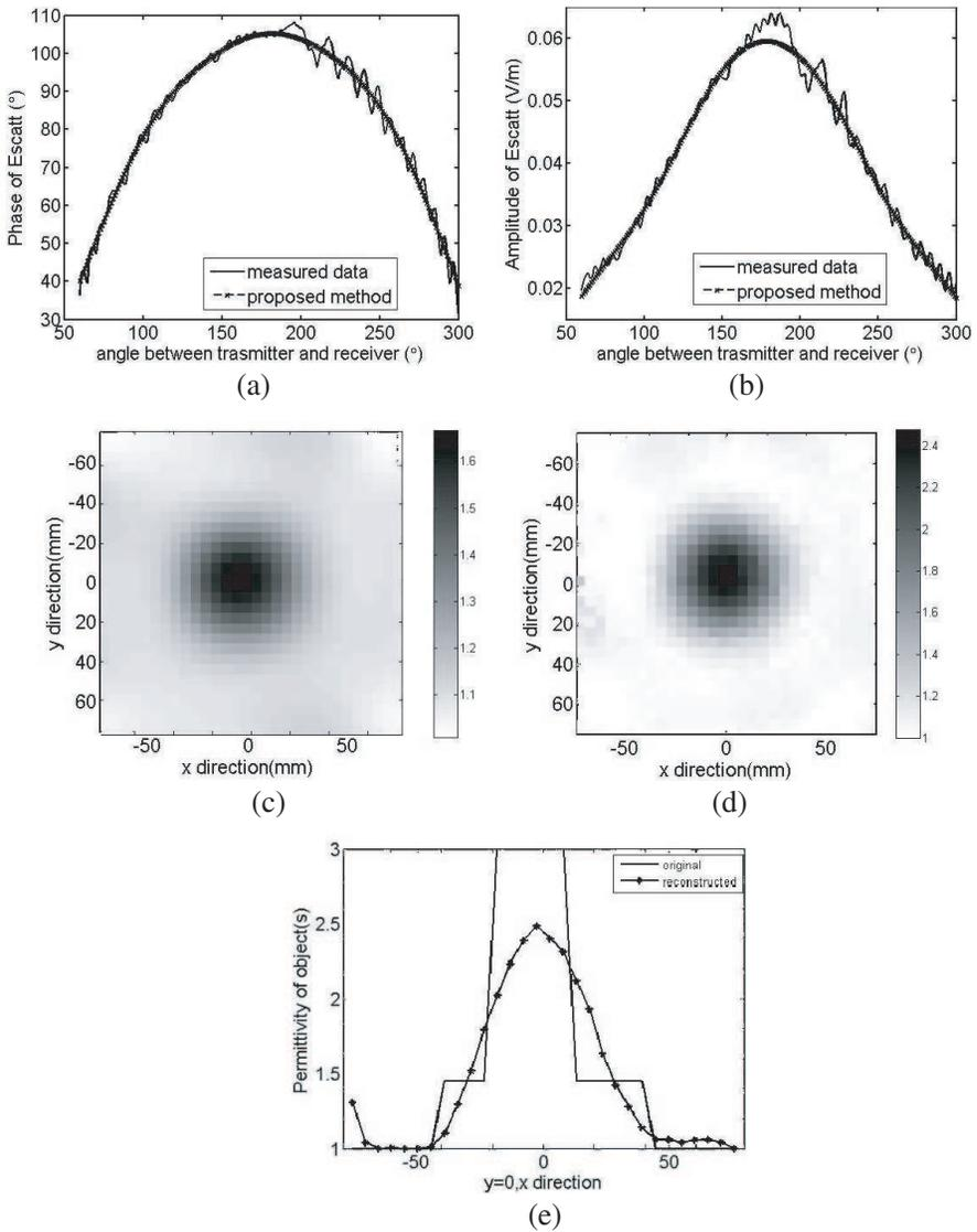
**Figure 5.** The reconstruction for probed objects shown in Fig. 2(a): (a) Phase of the scattered field ( $\theta_s = 0^\circ$ ), (b) amplitude of the scattered field ( $\theta_s = 0^\circ$ ), (c) contrast map of the objects estimated by radiating equivalent current, (d) contrast map of the objects estimated by all equivalent current, (e) relative permittivity on the line  $y = 0$ .
