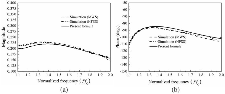
**Figure 4.** Aperture reflection coefficient at the open-end of the standard WR-34 waveguide without a flange. (a) Magnitude, and (b) phase.
