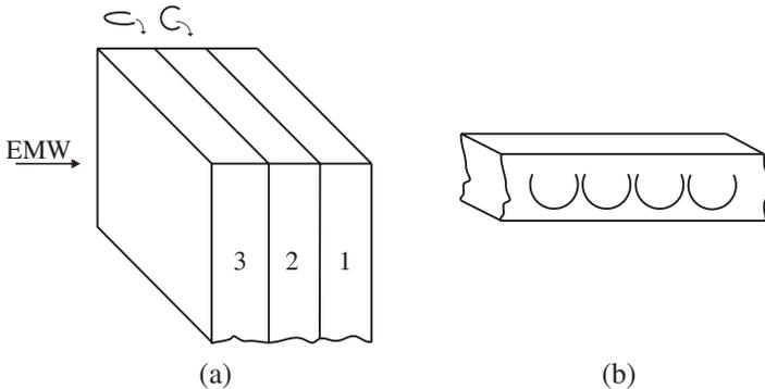
**Figure 4.** Low reflecting coating structure (a) and direct box with a dielectric array in the form of identically oriented flat open rings on one of its surfaces (b). 1 — absorber, 2 — layer composed of vertically glued dielectric parallelepipeds, 3 — layer that composed of horizontally bonded dielectric parallelepipeds (b).
