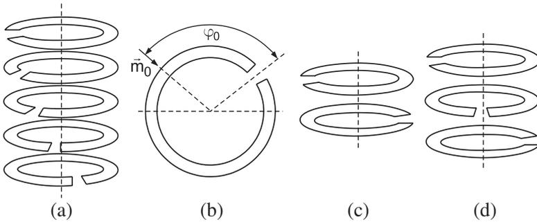
**Figure 1.** Chiral structure formed by disconnected rings.
