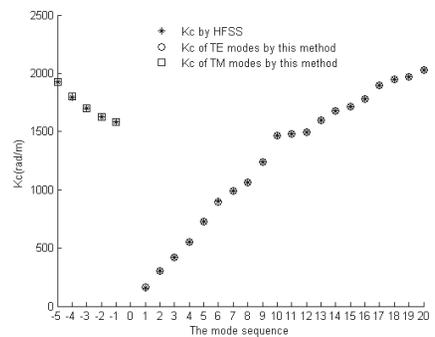
**Figure 9.** Cutoff wave numbers compared with HFSS.
