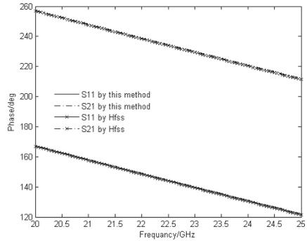
**Figure 6.** Phase compared with CAD software HFSS.
