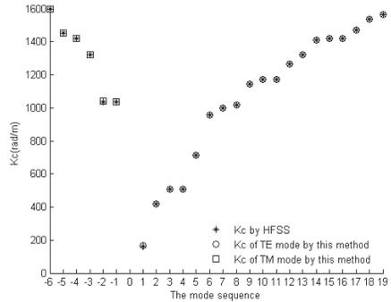
**Figure 4.** Cutoff wave numbers compared with HFSS.
