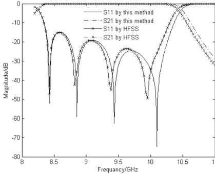
**Figure 10.** Magnitude compared with CAD software HFSS.
