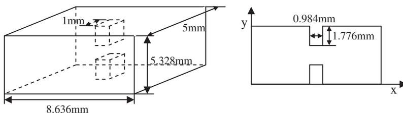
Figure 2. Double-ridged iris in rectangular waveguide.
