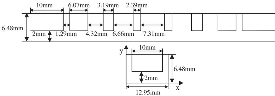
**Figure 7.** Rectangular single-ridged waveguide filter.
