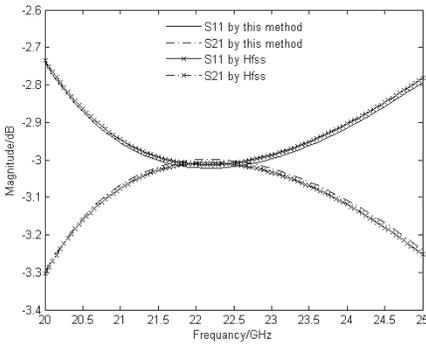
**Figure 5.** Magnitude compared with CAD software HFSS.
