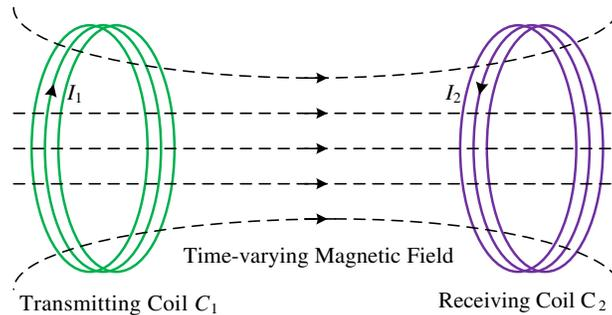
**Figure 1.** Basic model of wireless magnetic induction communication.
