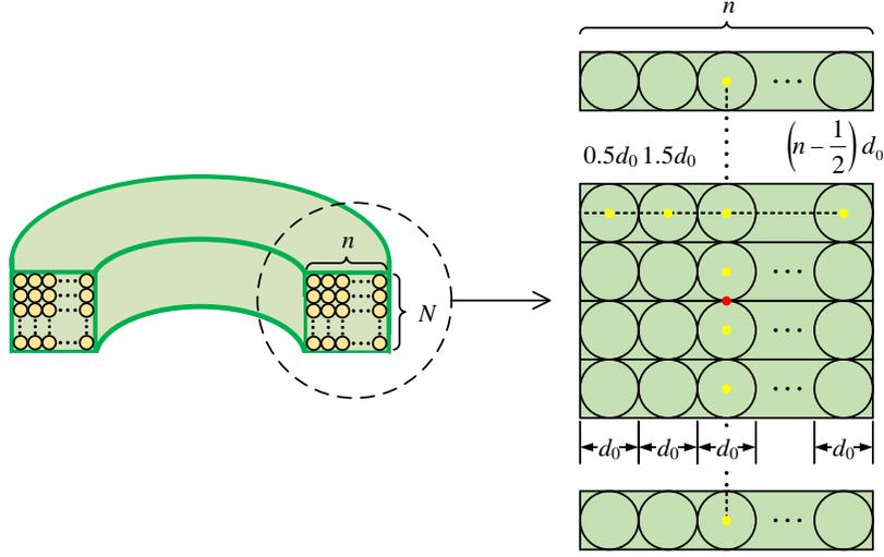
**Figure 5.** Rectangular cross-section with the radial turn  $n$ .
