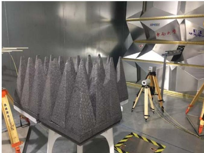
Figure 1. Measurement of the  $Q$  values of unloaded and loaded RC1.
