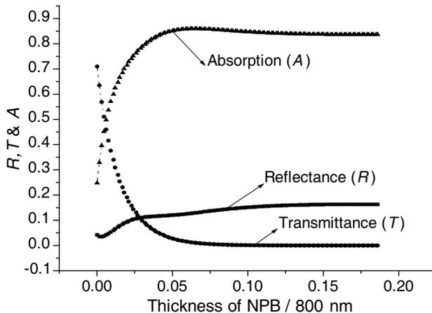
**Figure 8.**  $R$ ,  $T$  &  $A$  for metal-organic photonic crystals with air-substrate.
