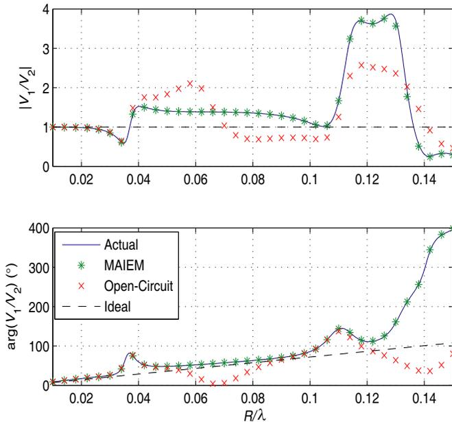
**Figure 3.** Wideband prediction of the amplitude ratio ( $|V_1/V_2|$ ) and phase difference ( $\arg(V_1/V_2)$ ) of the terminal voltages of two dipoles illuminated from the end-fire direction. Predictions are calculated using both the MAIEM and the open-circuit voltage method, the actual values are calculated using the MoM in the receiving mode, and the ideal values are those in the absence of mutual coupling.
