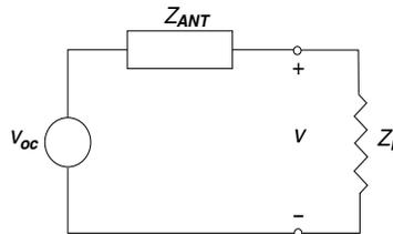
**Figure 1.** Equivalent circuit of a receiving antenna consisting of the equivalent open-circuit voltage,  $v_{oc}$ , the input impedance of the antenna,  $Z_{ANT}$ , the load impedance connected to the antenna,  $Z_L$ , and the terminal voltage  $v$  measured across the load impedance.
