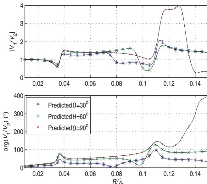
**Figure 4.** Wideband prediction of the amplitude ratio ( $|V_1/V_2|$ ) and phase difference ( $\arg(V_1/V_2)$ ) of the terminal voltages of two dipoles illuminated from three different elevation angles. The predicted values are calculated using the MAIEM and the actual values are calculated using the MoM in the receiving mode.
