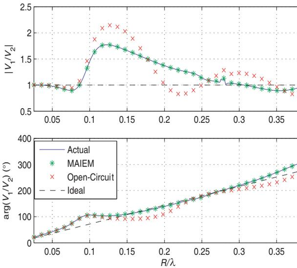
**Figure 7.** Wideband prediction of the amplitude ratio ( $|V_1/V_2|$ ) and phase difference ( $\arg(V_1/V_2)$ ) of the terminal voltages of two biconical elements illuminated from the end-fire direction. Predictions are calculated using both the MAIEM and the open-circuit voltage method, the actual values are calculated using the MoM in the receiving mode, and the ideal values are those in the absence of mutual coupling.
