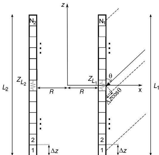
**Figure 2.** Array of two vertical wire elements of lengths  $L_1$  and  $L_2$ , discretized into  $N_1$  and  $N_2$  segments and centrally terminated into load impedances  $Z_{L_1}$  and  $Z_{L_2}$  respectively. The two elements are separated by a distance of  $2R$  and are illuminated by a signal having an elevation angle  $\theta$ .
