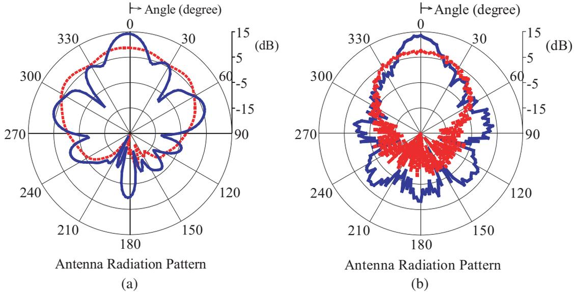
**Figure 8.** Radiation patterns of patch antenna with and without the artificial material. The artificial slab is set 30 mm in front of the patch antenna when it is used. (a) The simulated results. (b) The measured results.
