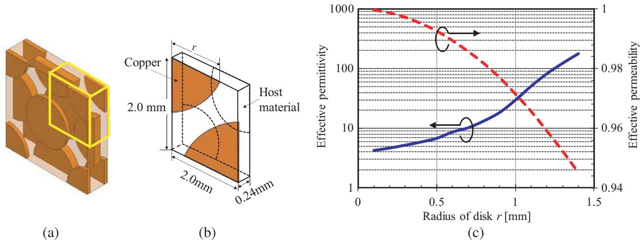
**Figure 2.** Analytical calculated result of an artificial material with the face-centered square (FCS) lattice structure. (a) A unit cell of FCS. (b) A quarter structure using a periodic boundary condition for simulation. (c) Calculated effective permittivity and permeability with respect to the radius  $r$  of a metal circular piece (6 conducting layers separated by FR-4 material, total thickness is 1.2 mm).
