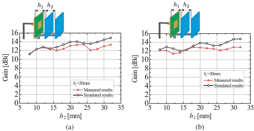
**Figure 9.** The simulated and measured gain with respect to the distance  $h_2$  when 2 slabs of the proposed artificial material are set in front of a patch antenna. (a)  $h_1 = 20$  mm. (b)  $h_1 = 30$  mm.
