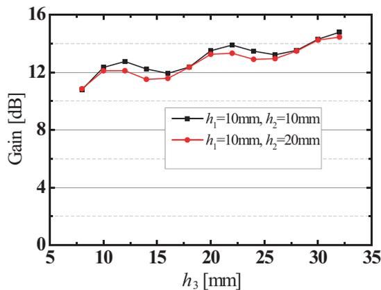
**Figure 10.** Gain enhancement when multiple slabs of the proposed artificial material are set in front of the patch antenna.
