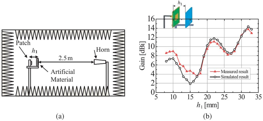
**Figure 7.** (a) Experimental setup for antenna gain evaluation. (b) The simulated and measured gain with respect to the distance  $h_1$  when one slab of the proposed artificial material is set in front of a patch antenna.
