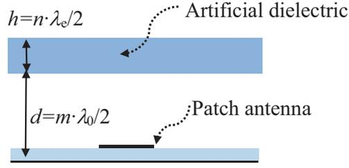
**Figure 3.** Structure of Resonant Cavity Antenna (RCA).
