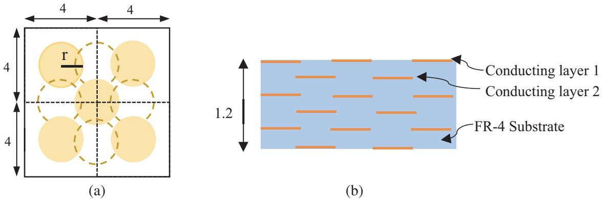
**Figure 4.** Structure of the proposed artificial material. Circular metal pattern  $r = 1.2$ , unit: mm. (a) Overview of 4-cells artificial material. The pattern in circle is on odd conducting layer, and the pattern in dot line circle is on even conducting layer. (b) Cross section view of partial artificial material.
