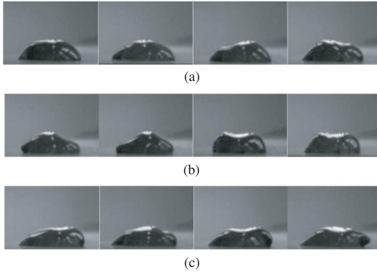
**Figure 2.** Three stages of water droplet motion under the AC field. (a) The first stage. (b) The second stage. (c) The third stage.
