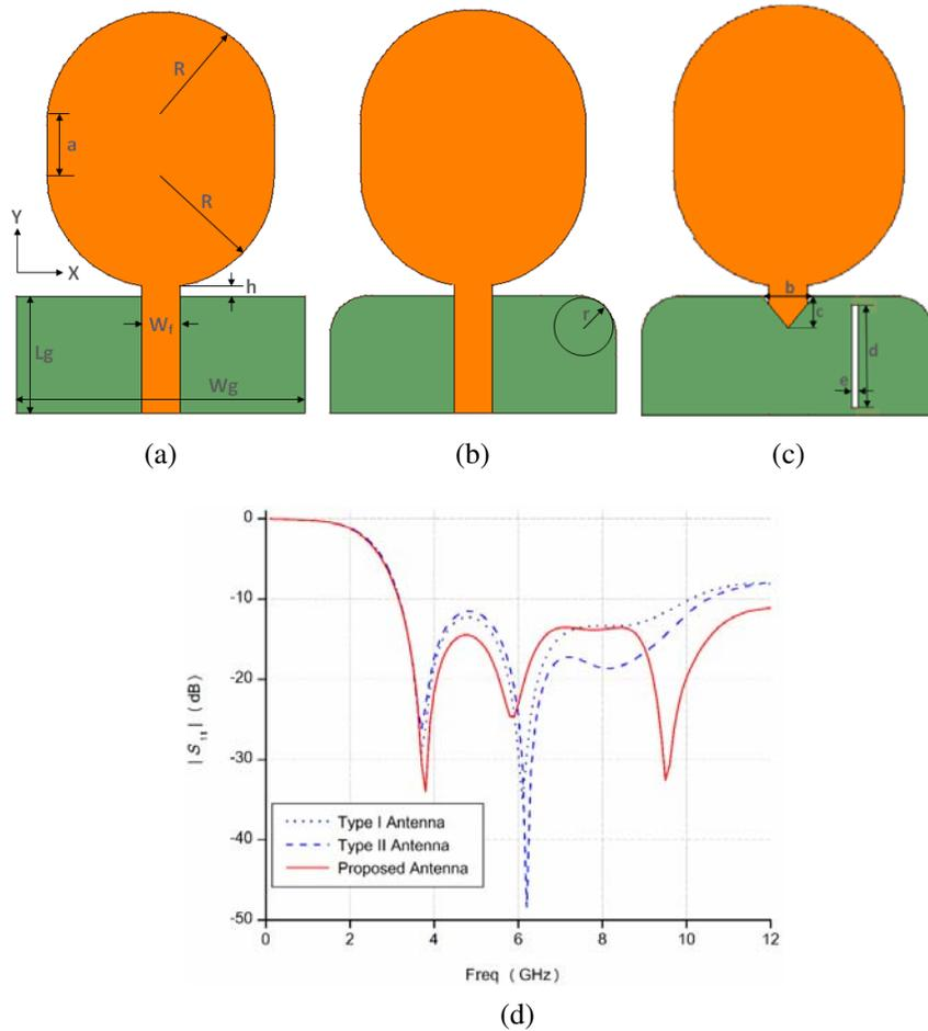
**Figure 1.** (a) Type I Antenna, (b) type II Antenna, (c) back view of the Proposed Antenna Type-III, (d) comparative frequency characteristics of the Type I, II and Proposed Antenna Type-III.
