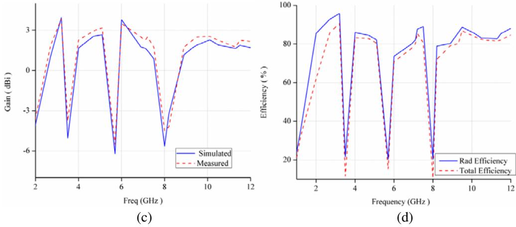
**Figure 4.** (a) Return loss curve plot, (b) VSWR curve plot, (c) gain curve plot, (d) simulated radiation and total efficiency plot.
