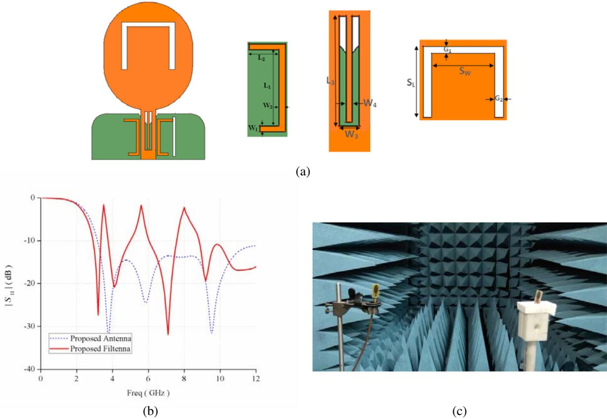
**Figure 2.** (a) Proposed Filtenna (and its components), (b) simulated return loss with frequency, (c) apparatus aligned to measure emission pattern from proposed filtenna in an anechoic chamber.
