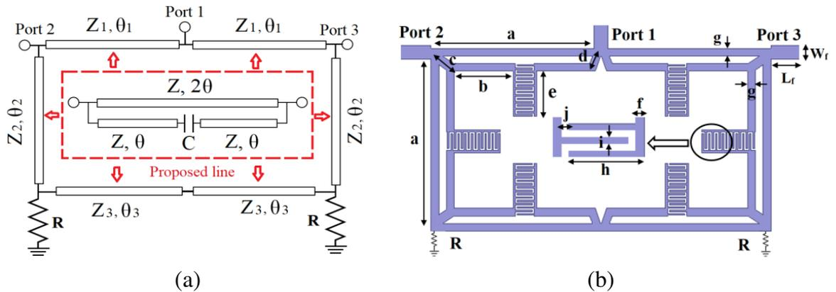
**Figure 3.** TL model and layout of GPD (a) TL model, (b) proposed GPD: with optimum value of  $L_f = 5$ ,  $W_f = 2.4$ ,  $a = 28.8$ ,  $b = 10.4$ ,  $c = 3.3$ ,  $d = 3.2$ ,  $e = 8$ ,  $f = 0.4$ ,  $g = 1.4$ ,  $h = 3$ ,  $i = j = 0.3$ , (dimensions are in mm),  $n = 16$ .
