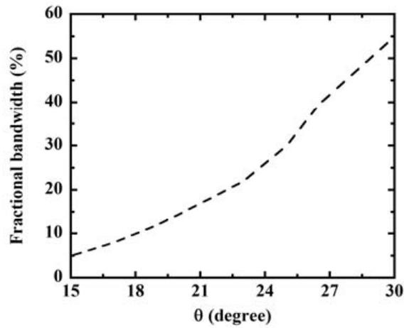
Figure 4. Variation of fractional bandwidth with  $\theta$  for  $Z_o = 70.7 \Omega$ , and  $f = 0.95$  GHz.
