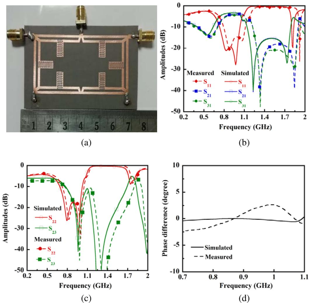
Figure 5.  $S$ -parameter responses of the GPD and fabricated unit: (a) Fabricated prototype, (b)  $S_{11}$ ,  $S_{21}$ ,  $S_{31}$ , (c)  $S_{22}$ ,  $S_{23}$ , (d) phase difference between output ports.
