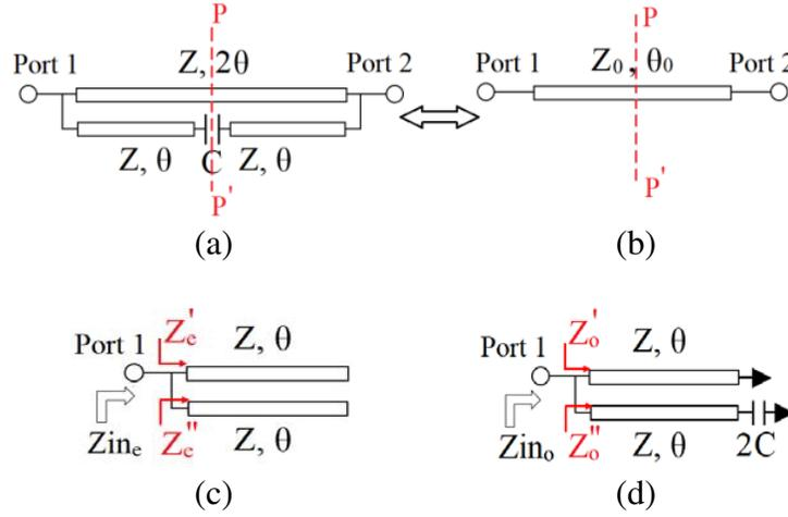
**Figure 1.** Conventional and proposed line: (a) Proposed, (b) conventional, (c) even mode, (d) odd mode.
