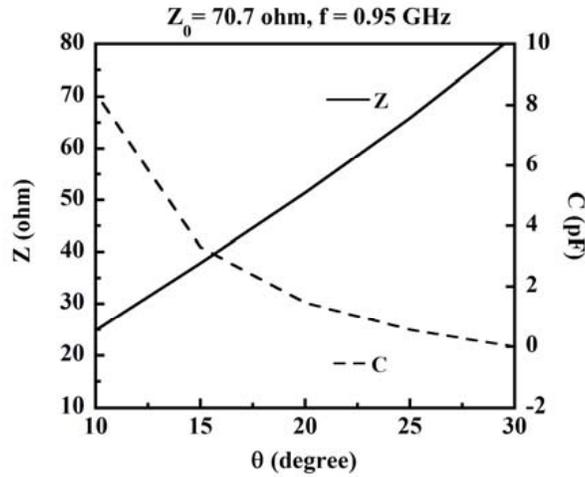
**Figure 2.** Variation of  $Z$  and  $C$  with  $\theta$  for  $Z_0 = 70.7 \Omega$ , and  $f = 0.95$  GHz for CDTL.
