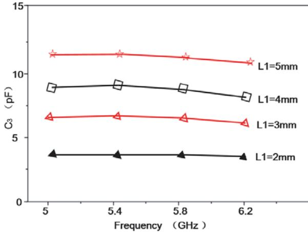
**Figure 4.** Capacitance  $C_3$  varies with the length  $L_1$ .
