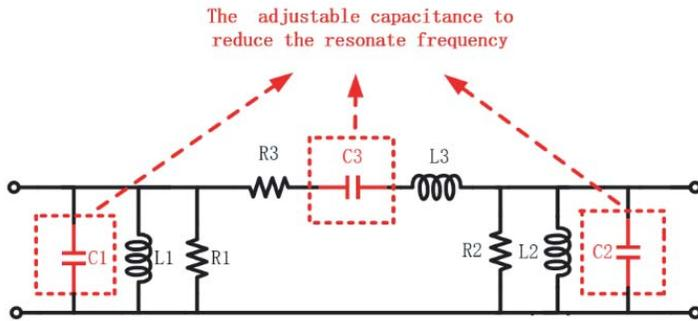
**Figure 2.** The equivalent circuit of the filter.
