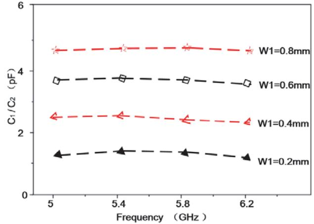
**Figure 5.** Capacitance  $C_1/C_2$  varies with the width  $W_1$ .
