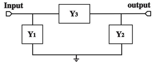
**Figure 3.** Simplified Y model of the filter.
