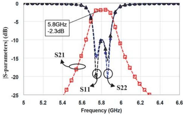
**Figure 8.** Measured  $S$  parameters of the filter.
