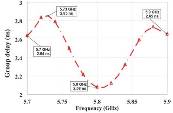
**Figure 9.** Measured group delay of the filter.
