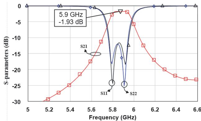
**Figure 6.** Simulated  $S$  parameters of the filter.
