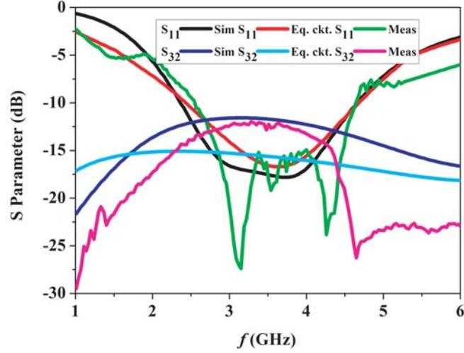
**Figure 5.** Isolation between two output terminals and return loss at input terminal.
