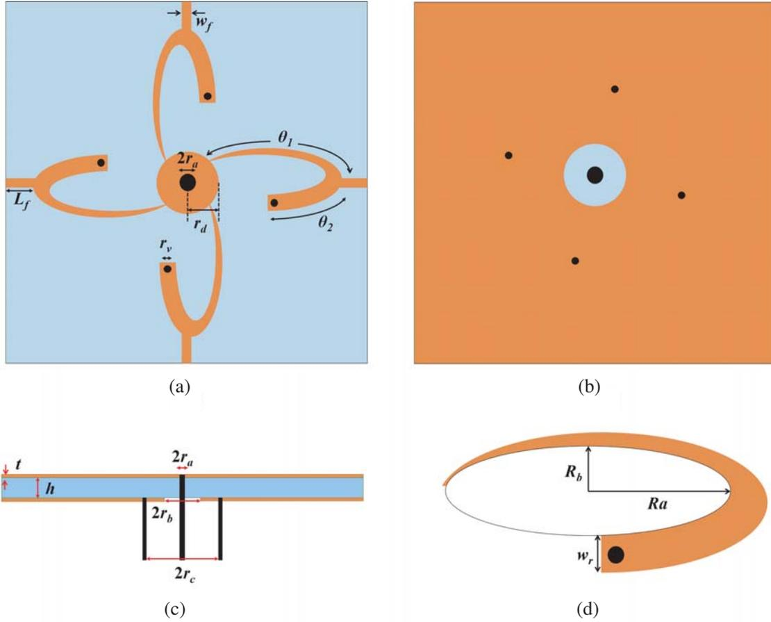
**Figure 2.** Configuration of the power divider, (a) top layer, (b) bottom layer, (c) cross-section, and (d) detailed view of an elliptical resonator.
