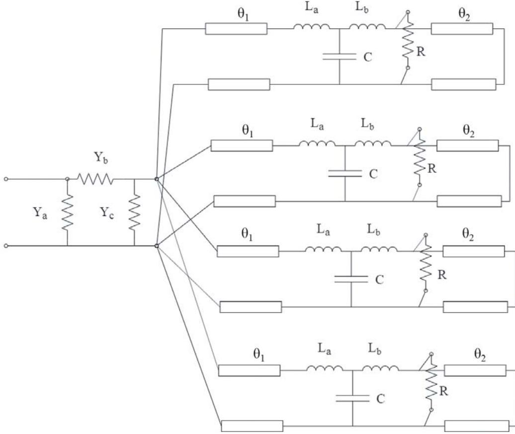
**Figure 3.** Equivalent circuit model of 4-way power divider.
