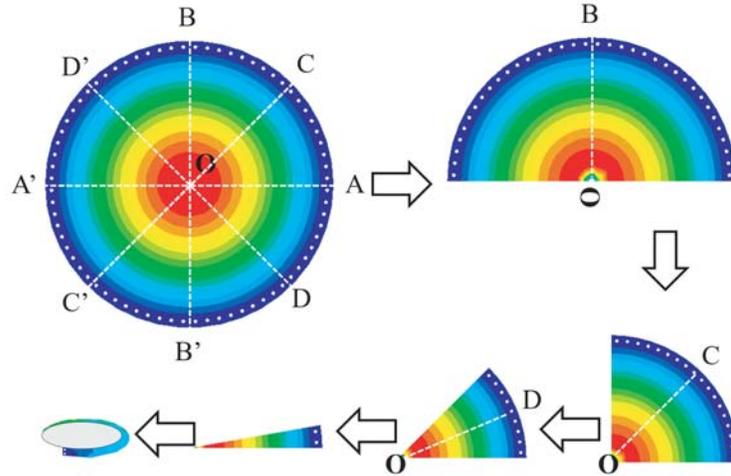
**Figure 1.** Evolution of elliptically curved SIW resonator.
