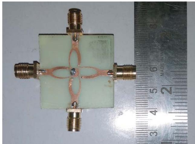
**Figure 4.** Photograph of the fabricated prototype.
