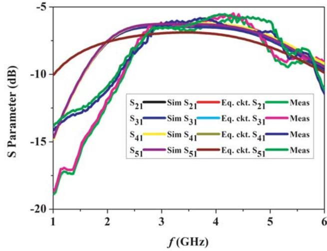
**Figure 6.** Insertion loss between input and output ports.
