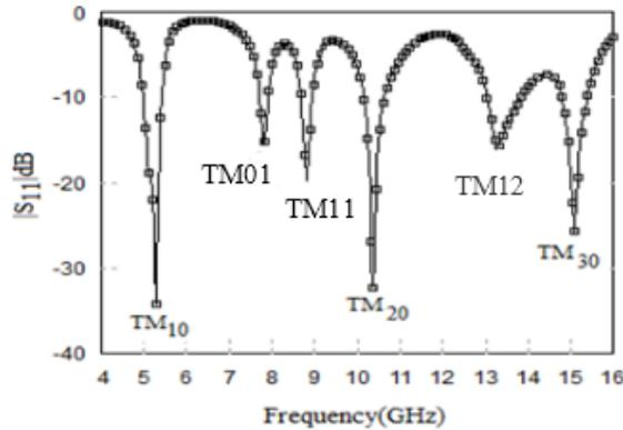
**Figure 3.** Simulated  $|S_{11}|$  characteristic of the reference array.
