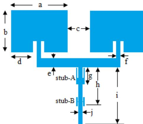
**Figure 1.** Structure of the proposed antenna array.
