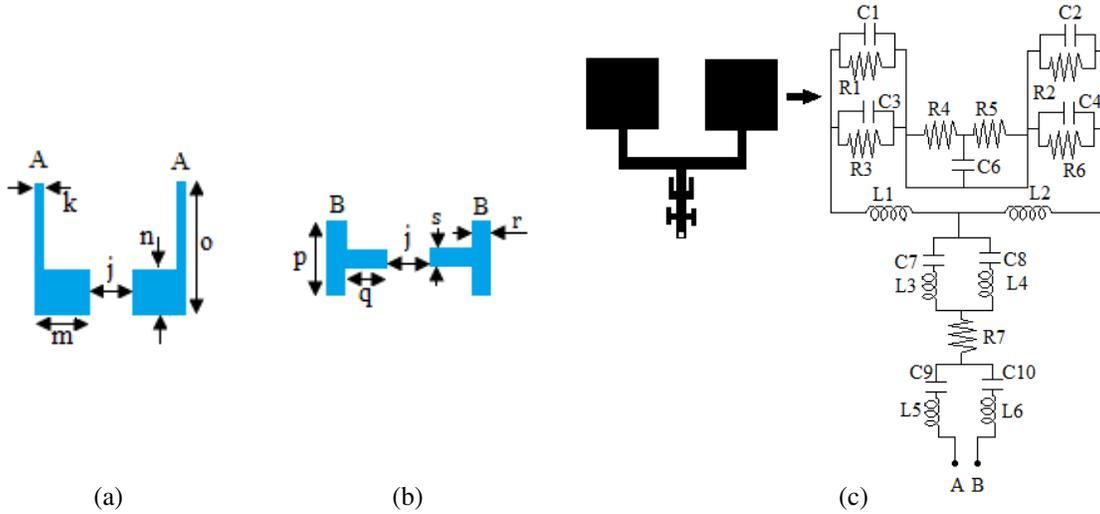
**Figure 2.** (a) Stub ‘A’ of vertical length ( $o \approx \lambda_{g1}/2$  ( $\lambda_{g1} \approx$  guided wavelength of the 1st harmonic frequency) and (b) Stub ‘B’ of vertical length ( $p \approx \lambda_{g2}/4$  ( $\lambda_{g2} \approx$  guided wavelength of 2nd harmonic frequency). (c) Equivalent circuit of stub integrated array.
