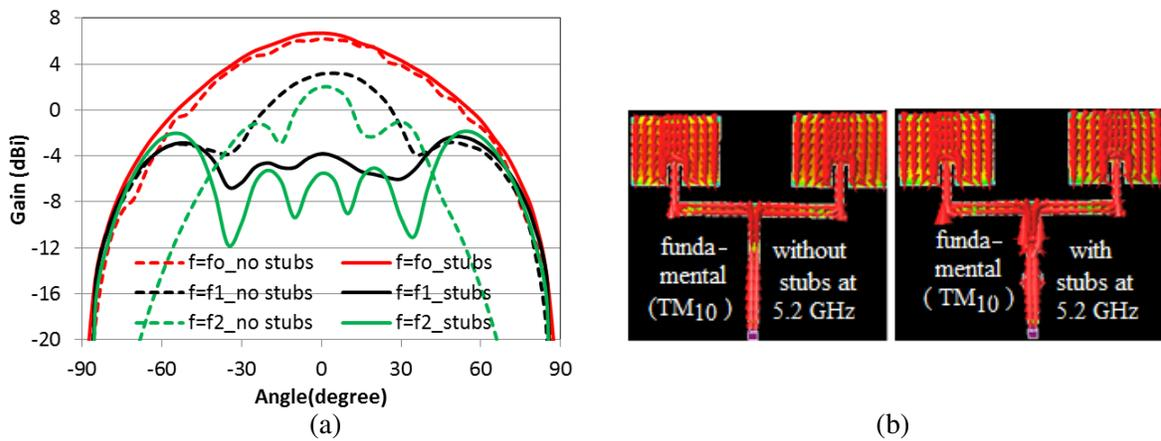
**Figure 6.** (a) Simulated elevation pattern views (co-pol.) of the array [ $f_0$  = fundamental,  $f_1$  = 1st harmonic and  $f_2$  = 2nd harmonic]. (b) Surface current distribution at 5.2 GHz (from left without stubs and with stubs).
