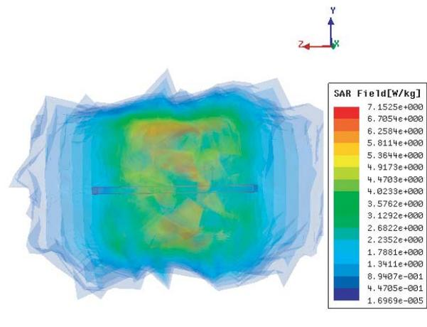
**Figure 6.** Simulated average SAR of the proposed antenna at 915 MHz.
