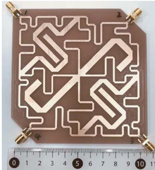
**Figure 6.** Photograph of fabricated microstrip dual-band crossover.
