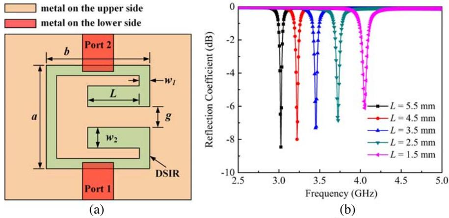
**Figure 2.** Resonance characteristic of the folded DSIR. (a) Geometrical layout. (b) Reflection coefficient. Other parameters are as follows:  $a = 7.0$  mm,  $b = 7.0$  mm,  $w_1 = 0.5$  mm,  $w_2 = 1.0$  mm, and  $g = 1.0$  mm.
