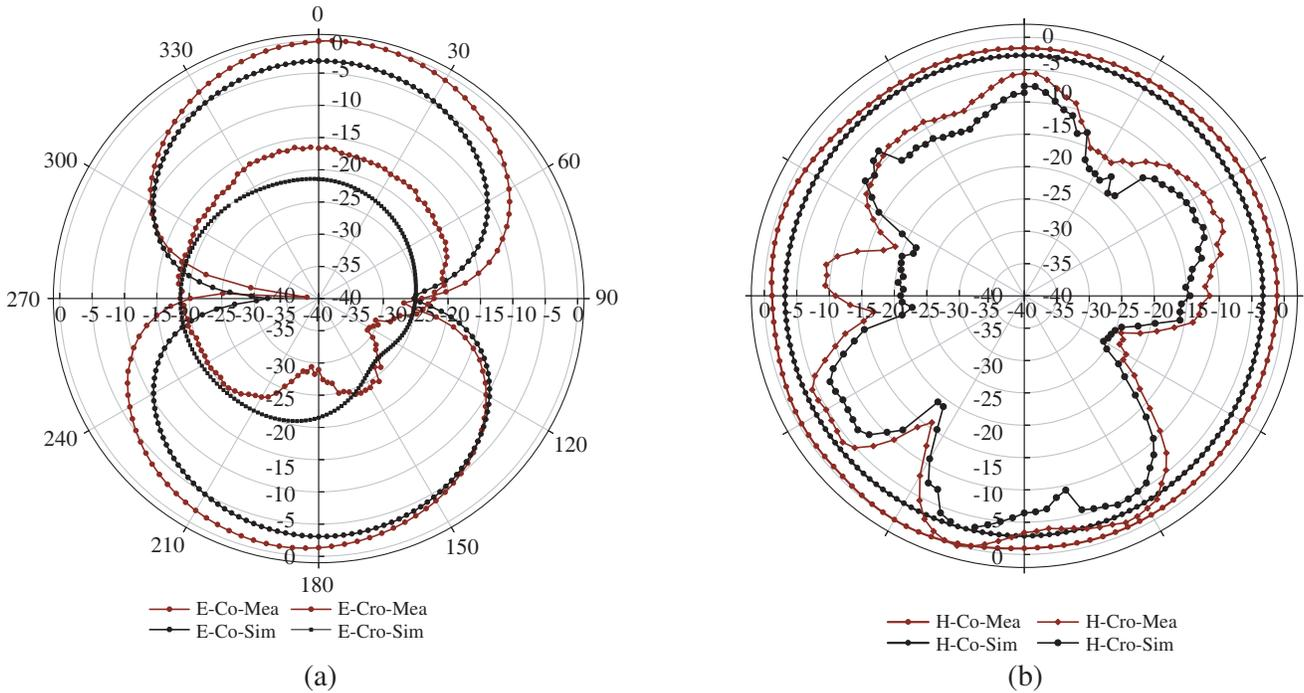
**Figure 6.** Simulated and measured radiation patterns of the proposed antenna at 1.22 GHz. (a)  $E$ -plane, (b)  $H$ -plane.
