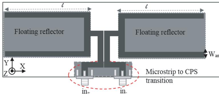
**Figure 2.** Layout of the standalone differential antenna with microstrip to coplanar strip line transition. The top copper layer is indicated in dark gray. The bottom copper layer is indicated in light gray.
