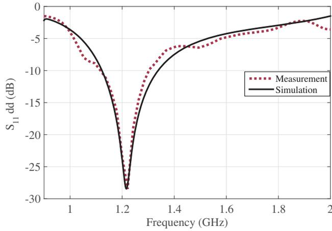
**Figure 5.** Return loss characteristics of the proposed antenna ( $l = 36$  mm,  $W_{ant} = 2$  mm,  $\epsilon_r = 4.4$ ,  $\tan \delta = 0.015$ , and  $h = 1.6$  mm).
