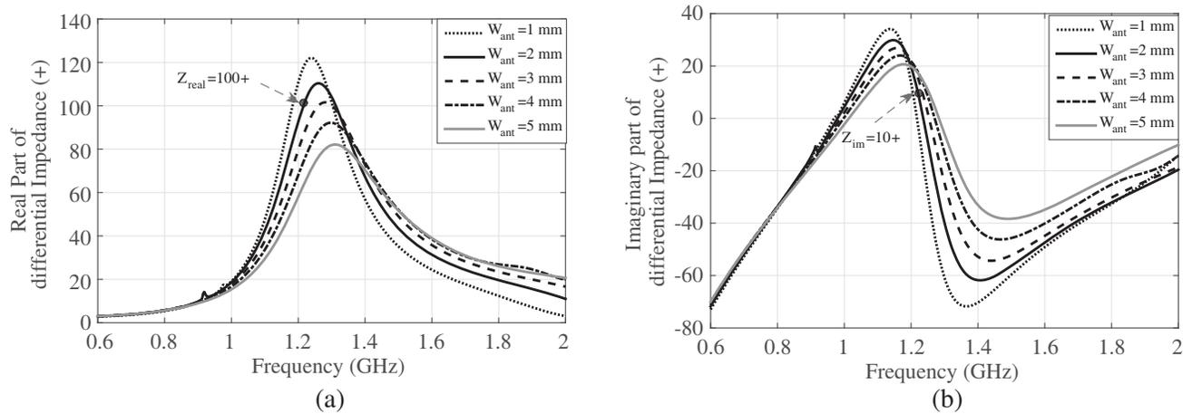
**Figure 3.** The (a) real and (b) imaginary parts of the differential impedance of the antenna for different arm widths  $W_{ant}$ . Dark line shows the proposed antenna.
