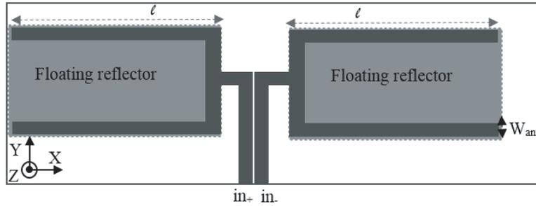
**Figure 1.** Geometry of the antenna. The top copper layer is indicated in dark gray. The bottom copper layer is indicated in light gray. ( $l = 36\ \text{mm}$ ,  $W_{ant} = 2\ \text{mm}$ ;  $\epsilon_r = 4.4$ ,  $\tan \delta = 0.015$ , and  $h = 1.6\ \text{mm}$ ).
