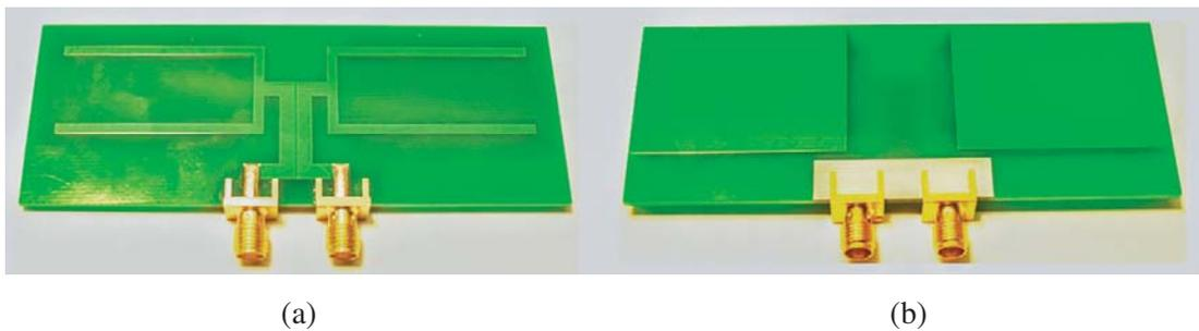
**Figure 4.** Differential antenna. (a) Front view, (b) back view.
