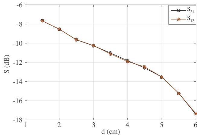
**Figure 8.** Power transfer curve of the proposed antenna as a function of distance  $d$ .
