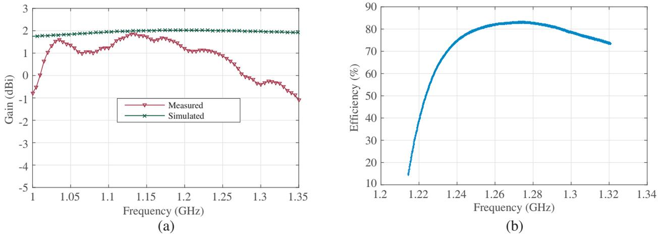
**Figure 7.** Gain and efficiency of the dipole antenna. (a) Simulated and measured gain of the dipole antenna, (b) measured efficiency of the dipole antenna.
