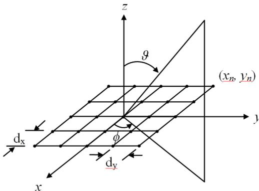
**Figure 1.** Geometry and notation of the considered planar, rectangular grid.
