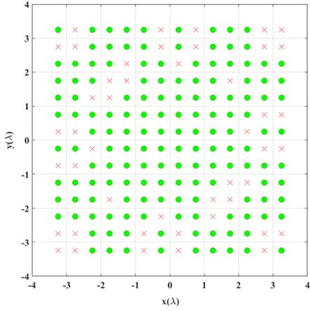
Figure 2. Array of 150 elements obtained in [5].
