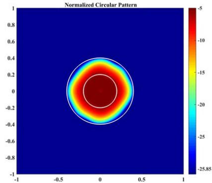
Figure 5. 2D circular pattern. The two white circles represent the mainlobe and sidelobe boundaries respectively.
