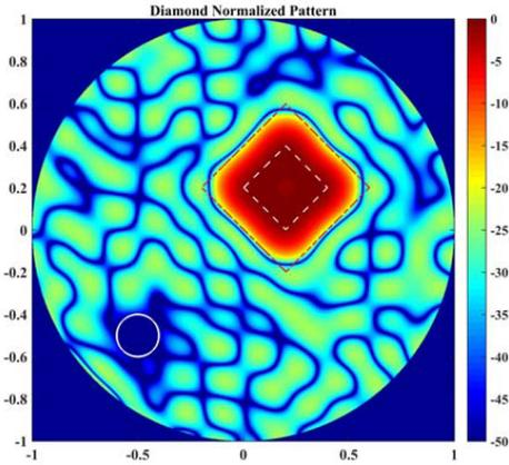
**Figure 8.** 2D diamond-shape pattern. The white circle and dashed square, together with the red dash-dotted square represent the null region, the mainlobe and sidelobe regions boundaries respectively.
