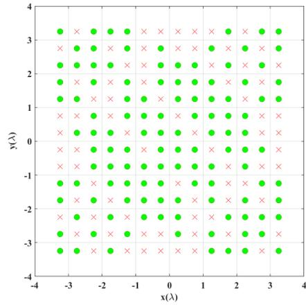
Figure 3. Array of 119 elements obtained by means of our proposed algorithms.
