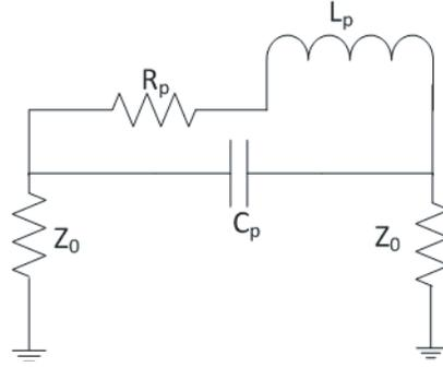
**Figure 1.** Equivalent circuit of the proposed DGS.
