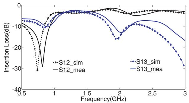
Figure 5. Simulated and measured insertion losses.
