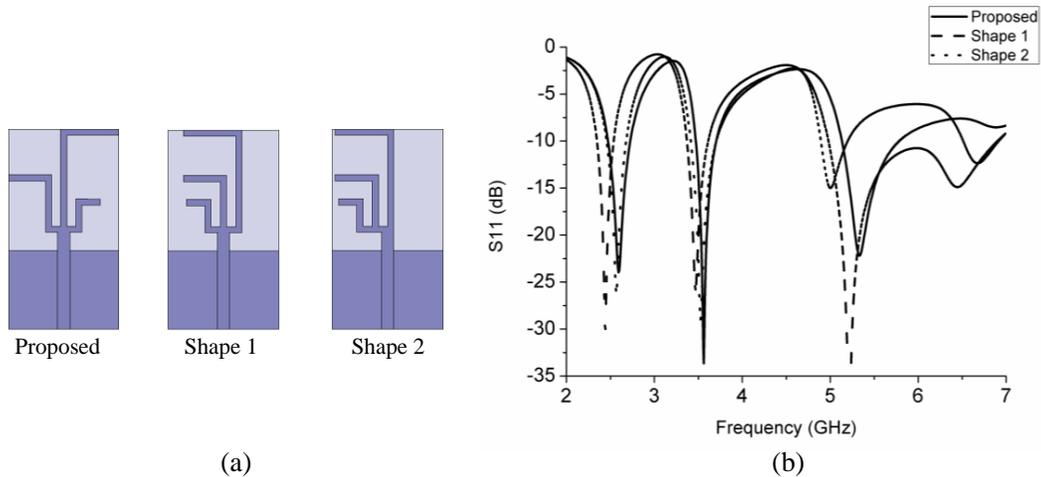
**Figure 3.** (a) Different antenna orientations and (b) their corresponding return losses.
