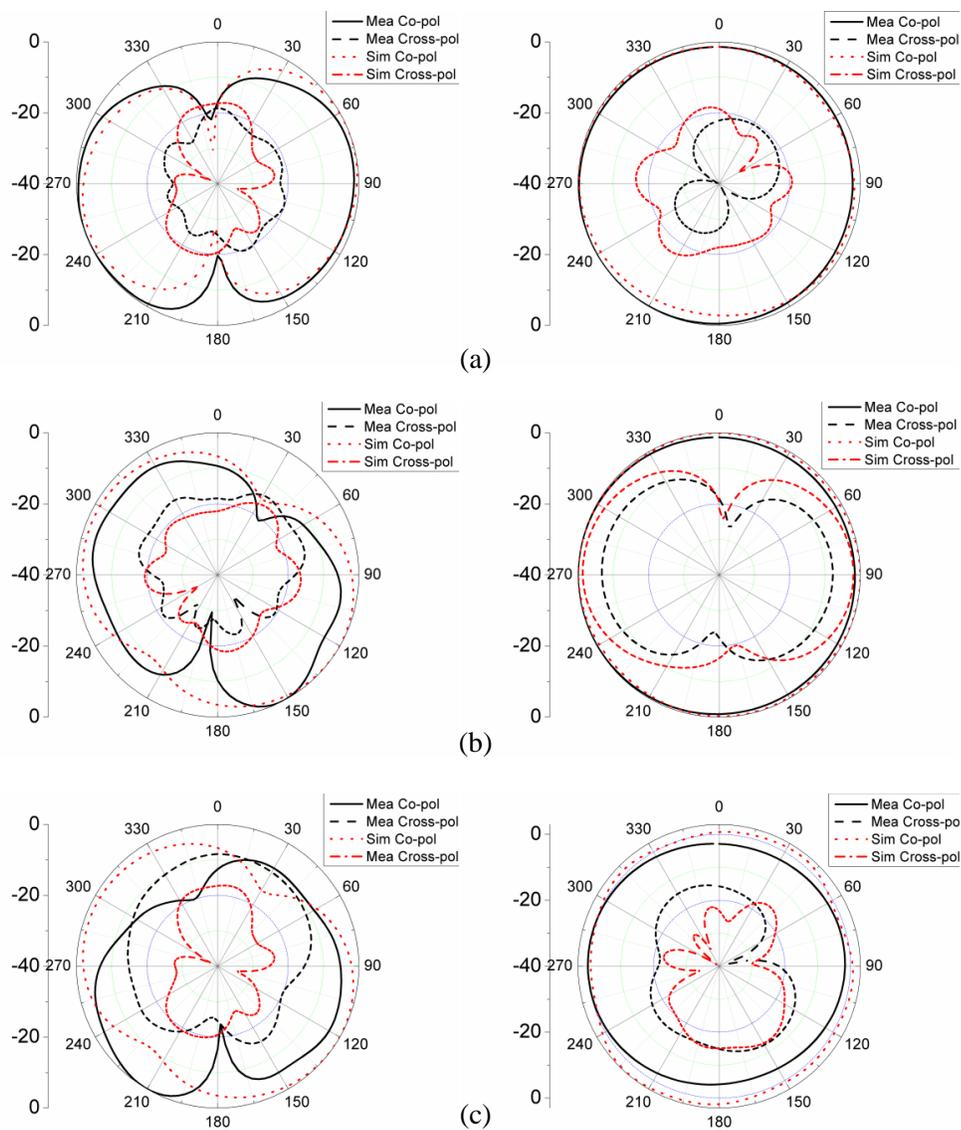
**Figure 8.** Measured (left) *E*-plane and (right) *H*-plane radiation patterns of the antenna at 2.5, 3.5, and 5.5 GHz.
