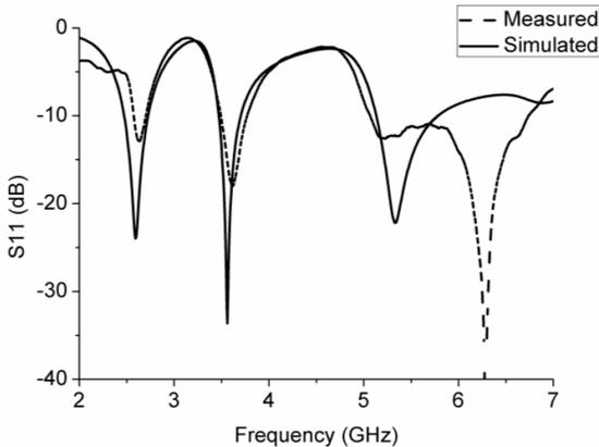
Figure 6. Measured return loss of the proposed antenna.
