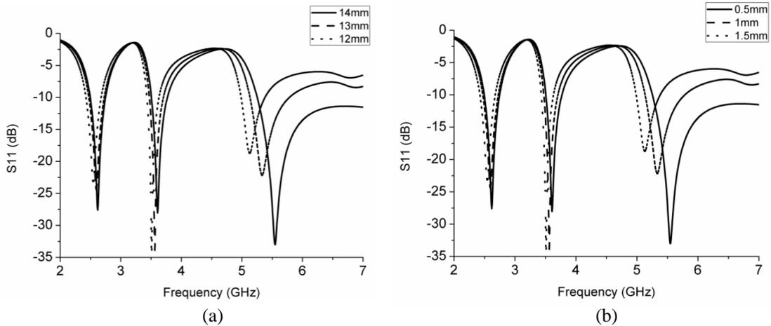
**Figure 2.** Simulated return loss for different; (a) ground plane heights, (b) gap between the L-shaped strips.
