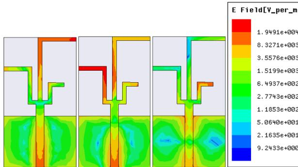
Figure 4. *E*-field distribution at 2.5 GHz, 3.5 GHz, and 5.5 GHz.
