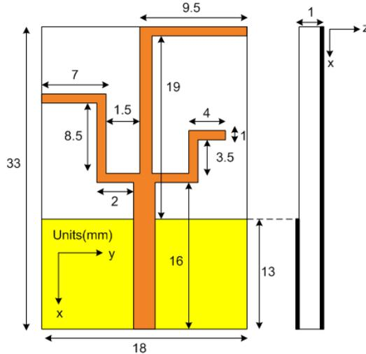
**Figure 1.** Geometry of the proposed antenna.
