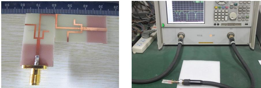
Figure 5. Photograph of the fabricated antenna with measurement setup.
