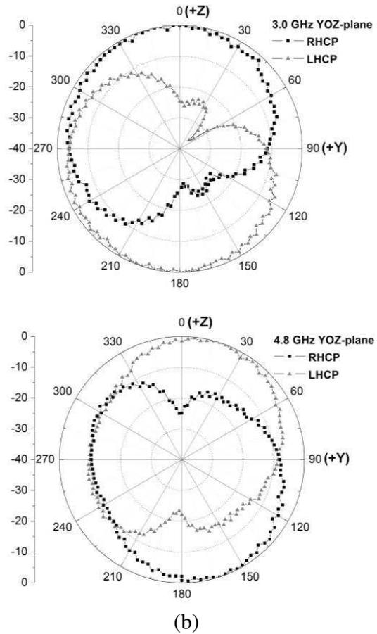
**Figure 8.** Measured radiation patterns of the proposed antenna at 3.0 GHz and 4.8 GHz. (a) *XOZ*-plane; (b) *YOZ*-plane.
