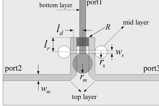
**Figure 1.** Configuration of the presented UWB power divider.
