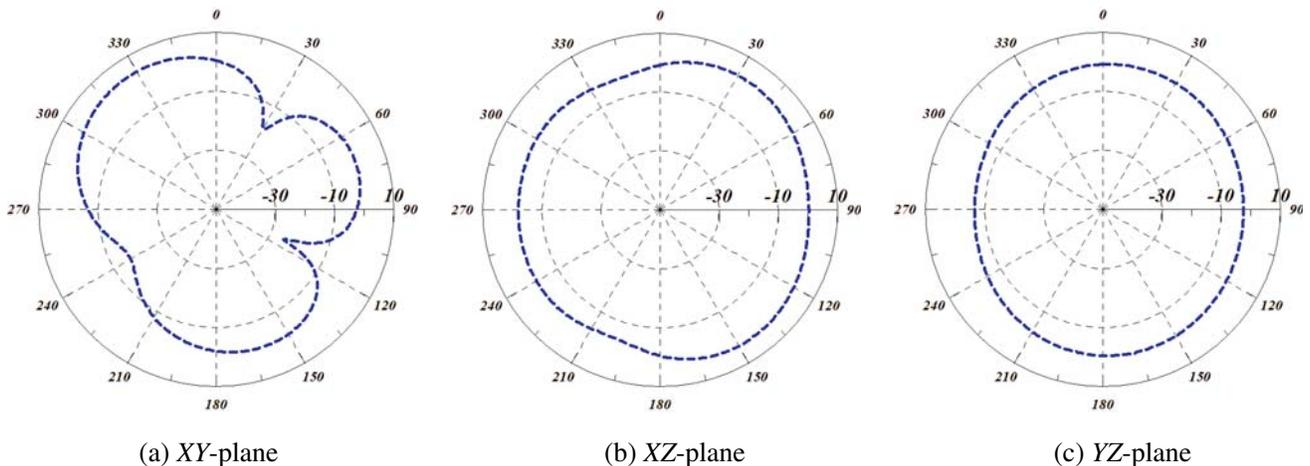
Figure 5. Measured radiation pattern of 2.45 GHz.
