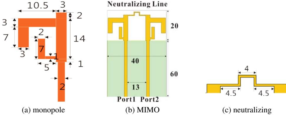
**Figure 1.** The structure of proposed MIMO (unit: mm).
