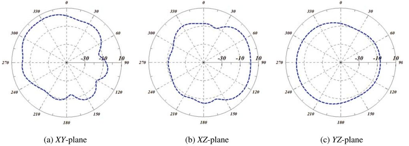
**Figure 6.** Measured radiation pattern of 5.2 GHz.
