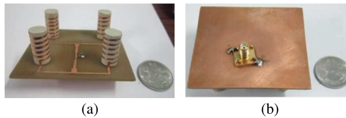
Figure 2. Photograph of fabricated antenna. (a) Top view. (b) Bottom view.
