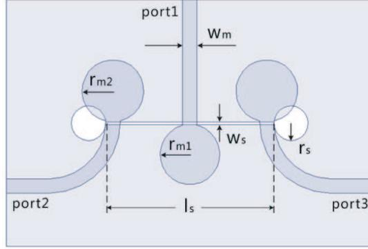
**Figure 1.** Configuration of the power divider.
