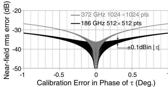
**Figure 3.** Sensitivity of the near-field solution to independent calibration errors in one of the two phase-shifter constants,  $\tau_{1,2}$ . Magnitude variations in  $\tau_{1,2}$  are  $\pm 0.1$  dB. Near-field data sets correspond to the AUT in [8].  $\sigma_2 = 0.001$ .
