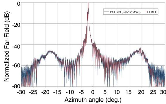
**Figure 5.** Predicted far-field of the 372 GHz 0.3 m diameter dual reflector antenna showing FEKO reference far-field and PSH (3H,  $0^\circ/120^\circ/240^\circ$ ) holographic reconstruction. SNR corresponds to 20 dB with respect to near-field beam peak.
