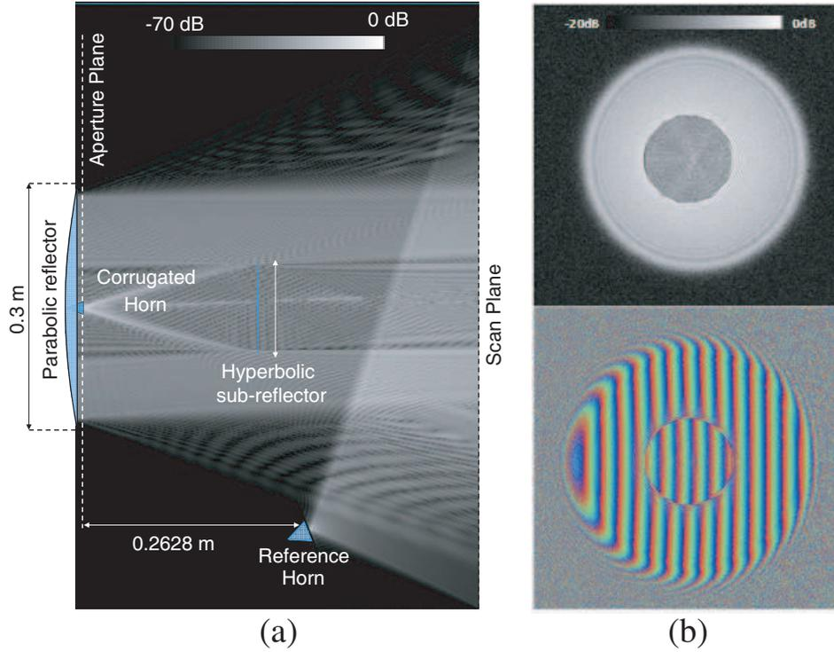
**Figure 4.** The back-propagated field of a 372 GHz 0.3 m diameter dual reflector antenna using FEKO to model the near-field and PSH (3H) for holographic reconstruction. (a) Horizontal axial plane reconstruction. In this case the near-field is noiseless. (b) Transverse reconstruction of the aperture plane focused at the sub-reflector plane. The near-field SNR is 20 dB with respect to near-field beam peak. The dimensions of the antenna are identical to those in [8].
