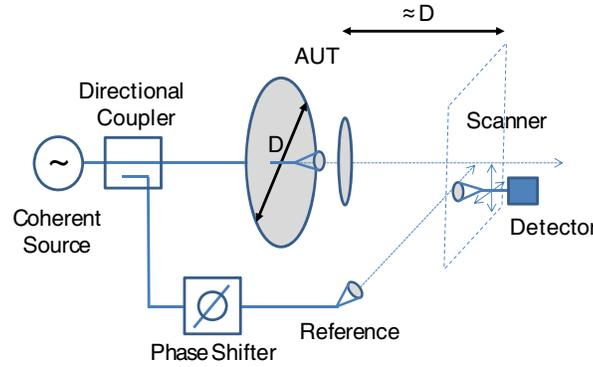
**Figure 1.** Proposed holographic system configuration for near-field antenna measurements. The reference horn is positioned to avoid illuminating the AUT.
