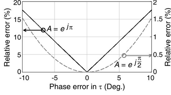
**Figure 2.** The calculated relative error in  $A$ , using either Equations (8) or (9), is shown as a function of the calibration error in the phase shifter  $\tau$ . The two extreme cases show the asymmetric nature of this error in the complex plane.
