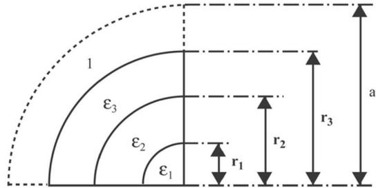
**Figure 2.** Cross sectional view of a multi-shells lens [7].
