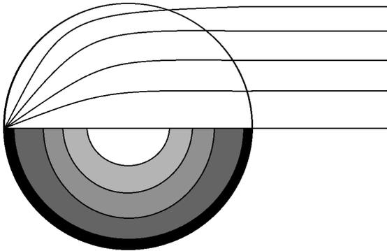
**Figure 1.** Ray tracing inside a Luneburg lens.
