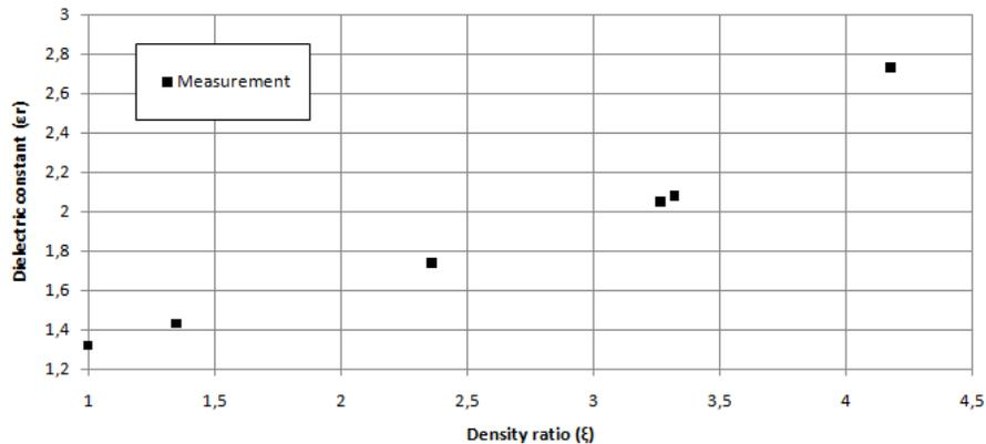
**Figure 5.** Dielectric constant versus density ratio  $\xi$  of the foam.
