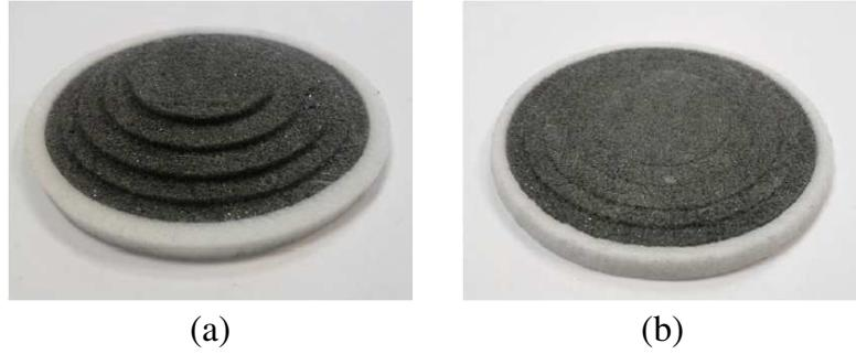
**Figure 6.** (a) Foam lens before and (b) after being pressed with the external Rohacell ring.
