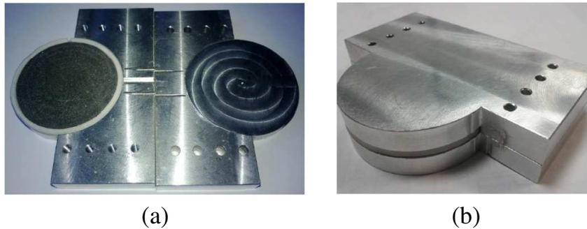
**Figure 7.** Lens in its (a) opened mechanical part and (b) closed mechanical part.
