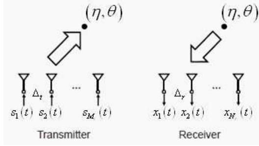
**Figure 1.** Monostatic MIMO noise radar scenario.
