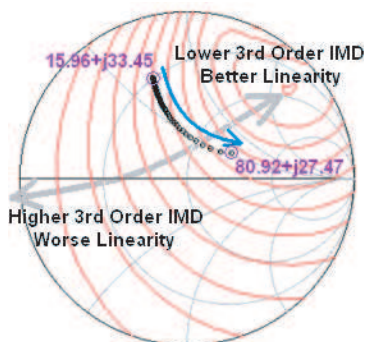
Figure 5. Third order IMD contours generated from load-pull simulation of the common emitter HBT transistor X2 (in Figure 1). Load impedances of X2 for C1 values ranging from 10 pF to 0.25 pF in steps of -0.05 pF are shown. The contour step size is 1 dB.
