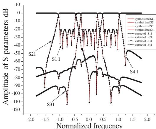
**Figure 4.** Attenuation and return loss of the triplexer.
