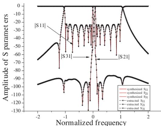
**Figure 3.** Attenuation and return loss of the duplexer.
