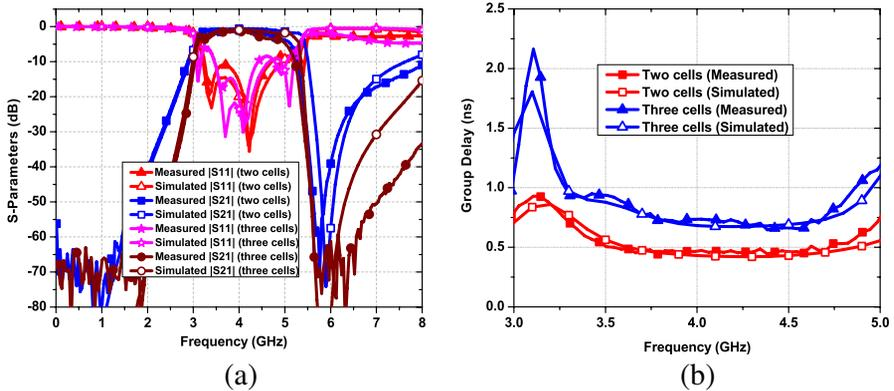
**Figure 7.** Simulated (HFSS) and measured characteristics of UWB bandpass filters with two and three unit cells. (a)  $S$  parameters and (b) group delay.
