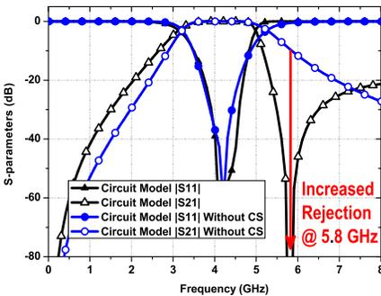
**Figure 2.** Simulated  $S$  parameters of the CRLH unit cell with and without  $C_S$ .
