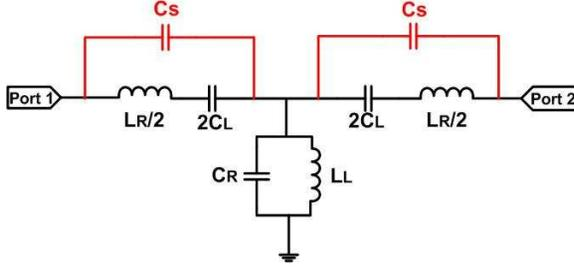
**Figure 1.** Circuit schematic of the proposed CRLH unit cell with  $C_S$ .
