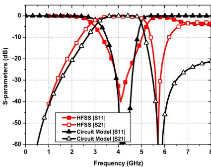
**Figure 5.** Simulated (HFSS and ADS)  $S$  parameters of the modified unit cell.
