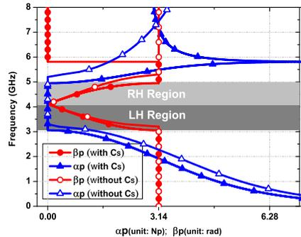
**Figure 3.** Dispersion/attenuation diagram of the proposed CRLH structure.
