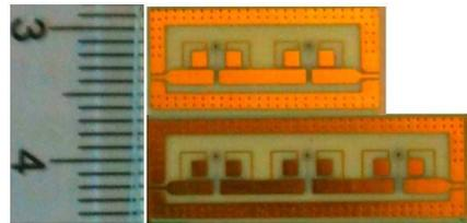
**Figure 6.** Photograph of the fabricated CRLH UWB bandpass filter with two (top) and three (bottom) unit cells.
