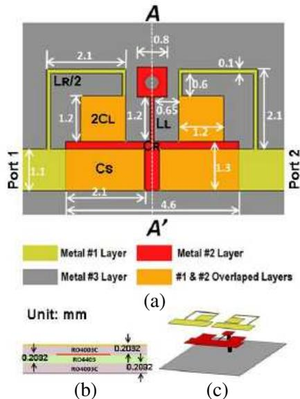
**Figure 4.** Illustration of the unit cell of proposed CRLH UWB bandpass filter. (a) Top view (it is symmetrical along the  $AA'$  line), (b) cross sectional view, and (c) 3-D explored view.
