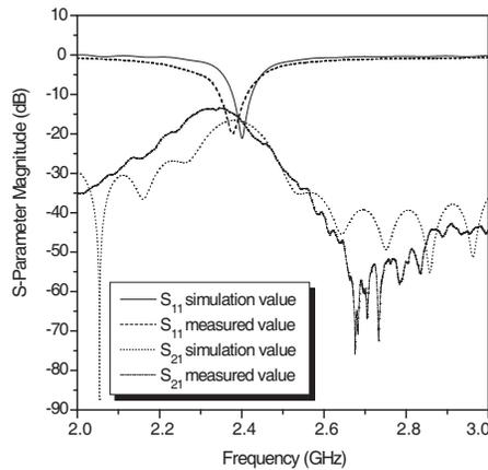
**Figure 3.** Measured and simulated  $S$ -parameter for the patch.
