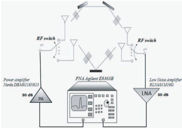
Figure 4. Measurement setup.
