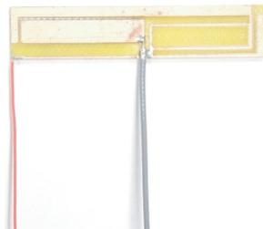
**Figure 2.** Photo of a design example fed by a 50-Ω mini-coaxial cable.
