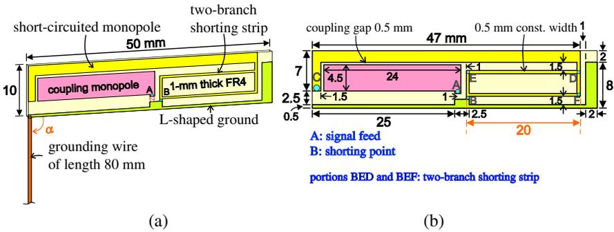
**Figure 1.** (a) Geometry of the compact, printed penta-band antenna for WWAN operation. (b) Detailed dimensions of the proposed antenna.
