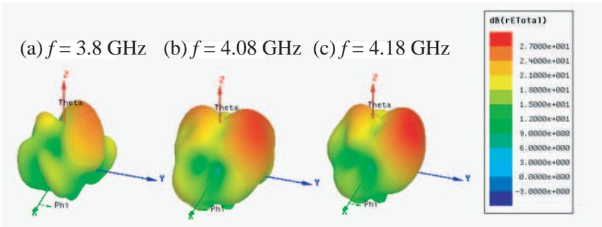
**Figure 5.** Computed radiation patterns (in dB) of the complete filtenna at different frequencies (corresponding to three reverse bias voltages). (a)  $f = 3.8$  GHz. (b)  $f = 4.08$  GHz. (c)  $f = 4.18$  GHz.
