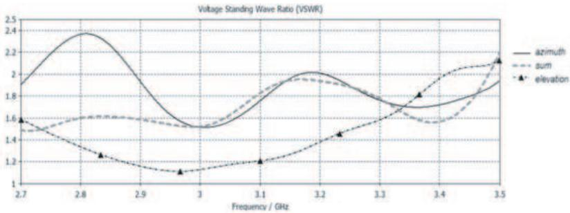
**Figure 7.** VSWR of the ports of the first monopulse antenna.
