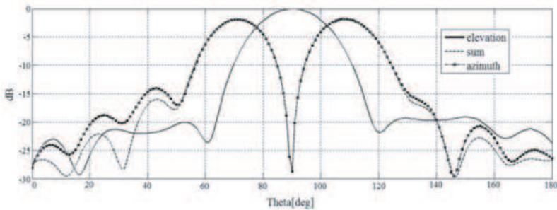
**Figure 8.** Radiation patterns of the first monopulse antenna.
