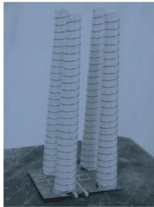
**Figure 10.** Prototype of the proposed antenna.
