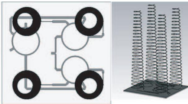
**Figure 6.** The first monopulse antenna with 4 conical helix antennas.
