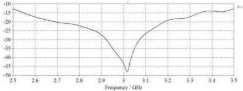
Figure 4. Return loss of the conical helix with microstrip matching line.
