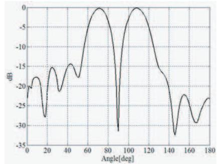
Figure 15. Measured *E*-plane difference pattern.
