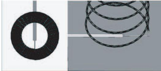
Figure 3. Conical helix antenna matched to microstrip line.
