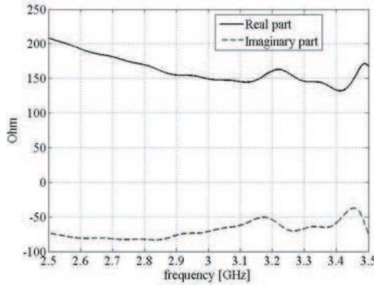
Figure 2. Input impedance of the designed conical helix antenna.
