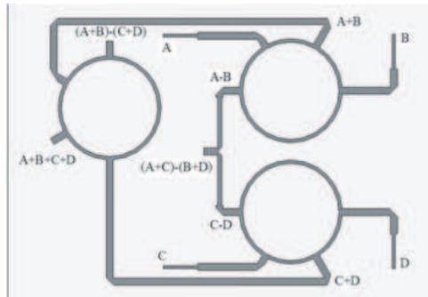
**Figure 5.** Monopulse comparator type I.
