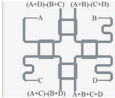
**Figure 9.** Monopulse comparator type II.
