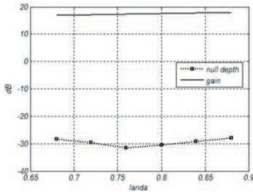
**Figure 16.** Gain and null depth versus space between the antennas.
