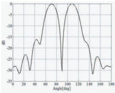
Figure 14. Measured *E*-plane difference pattern.
